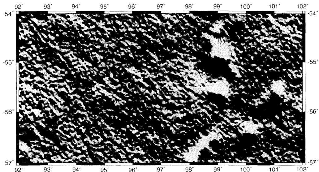
Fig. 9. Gravity anomaly images of sea mounts located at  $100^{\circ}\text{E}$ ,  $55^{\circ}\text{S}$  (raw 10 Hz data).
