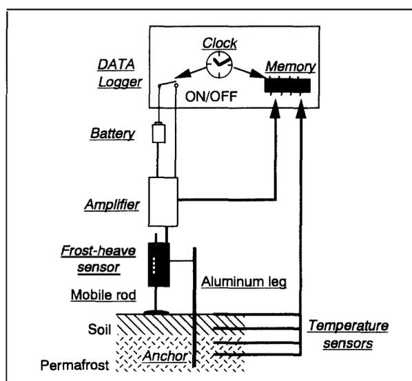
Fig. 4. Schematic sketch of the instruments.
