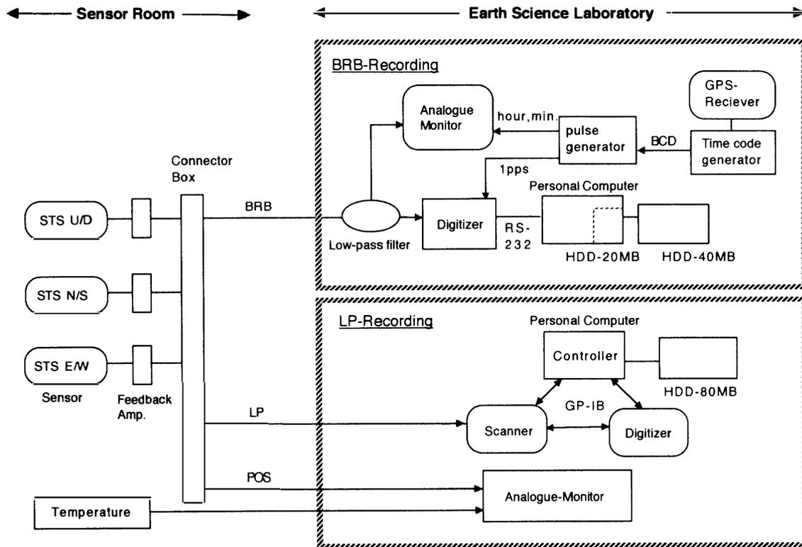
Fig. 3. Block diagram of STS recording system at Syowa Station. Upper figure : BRB-recording system ; Lower figure : LP-recording system.
