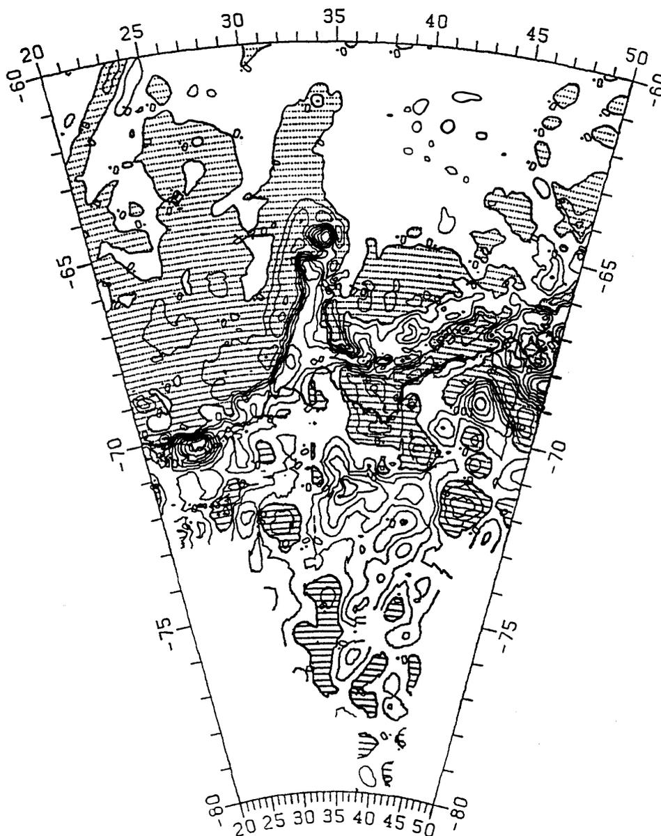
Fig. 3. Estimated gravity anomaly. Contour interval is 20 mgal.
