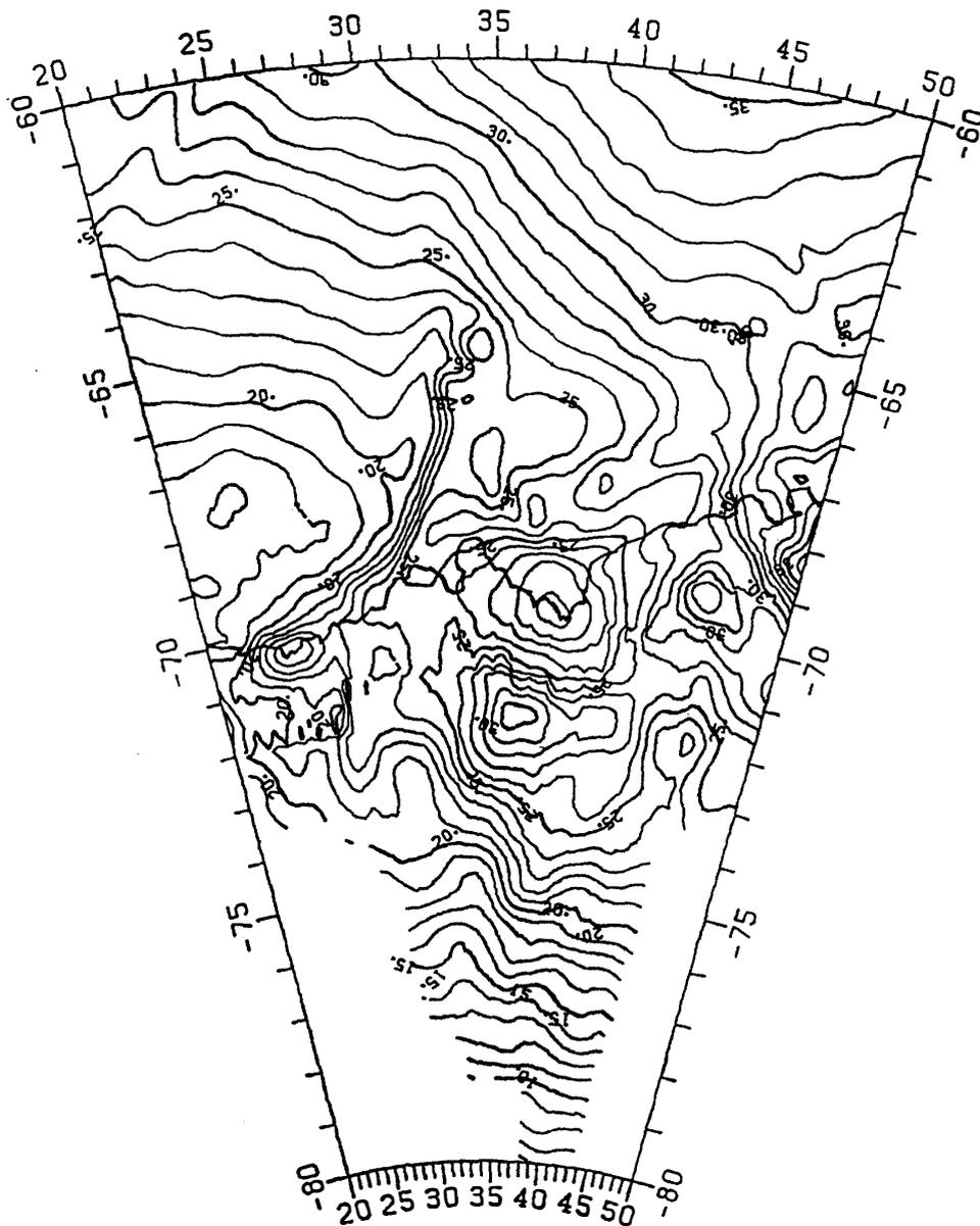
Fig. 4. Estimated geoidal undulation. Contour interval is 1 m.
