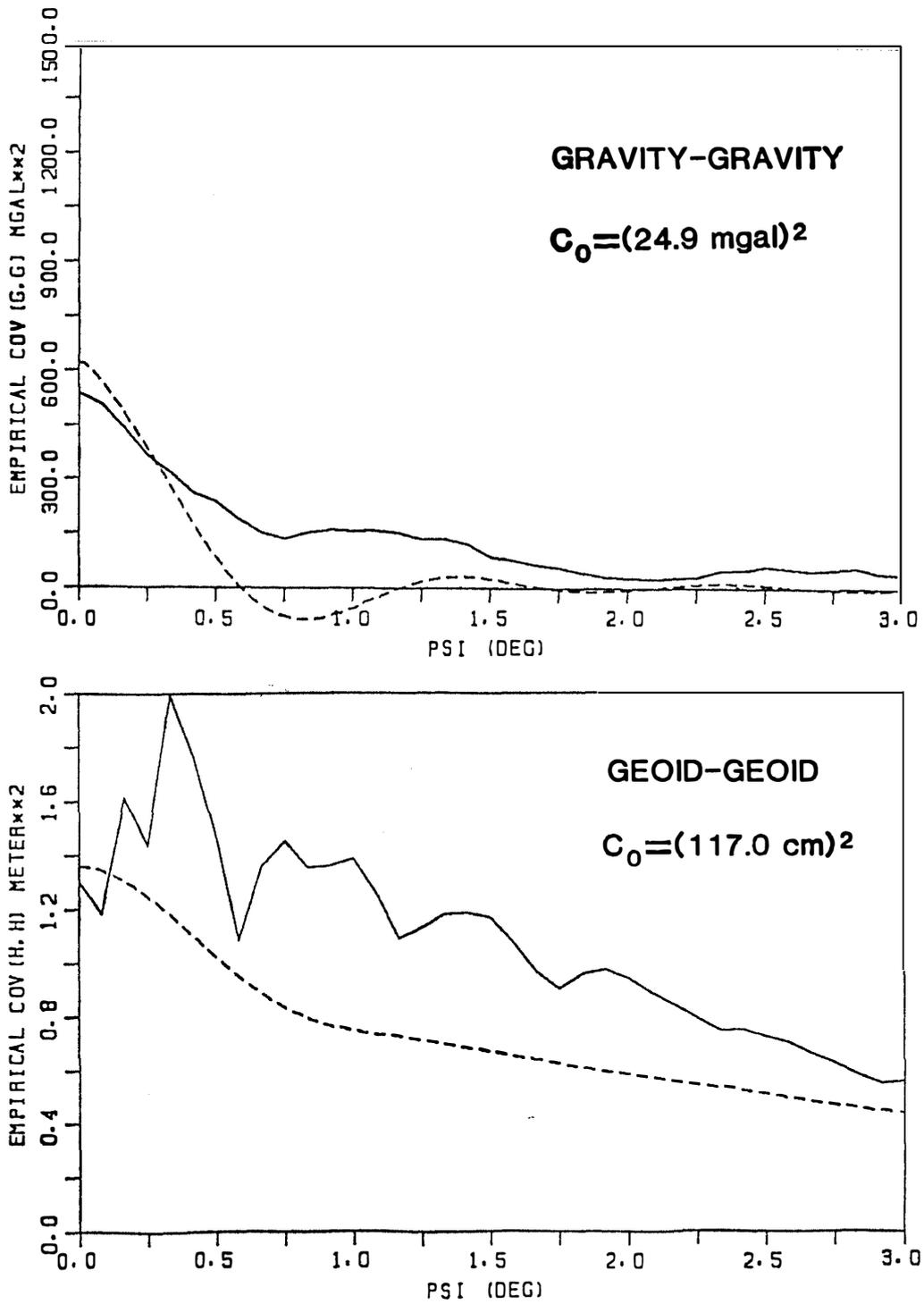
Fig. 2. Empirical (solid line) and synthesized (broken line) covariance functions.
