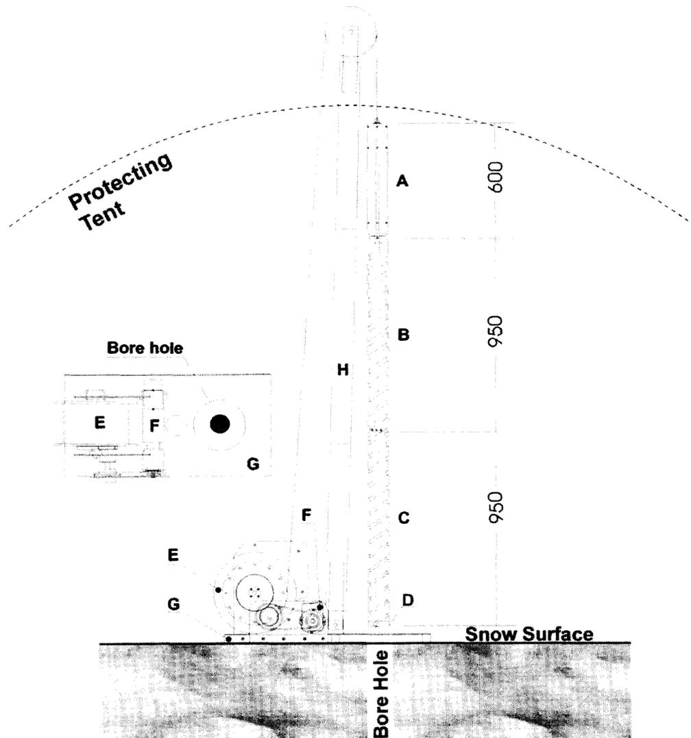
Fig. 2. The main components of the drill: A—the drive unit with motor and anti-torque system, B—the short chips barrel with the spiral allowing transport of the chips to the two openings on the top of the barrel, C—the core barrel, D—one piece cutting ring, E—winch with cable, F—winch motor, G—winch base plate and H—the 3 pieces of the tower installed inside the protective tent, (size in mm). Insert: view from the top onto the winch base plate.
