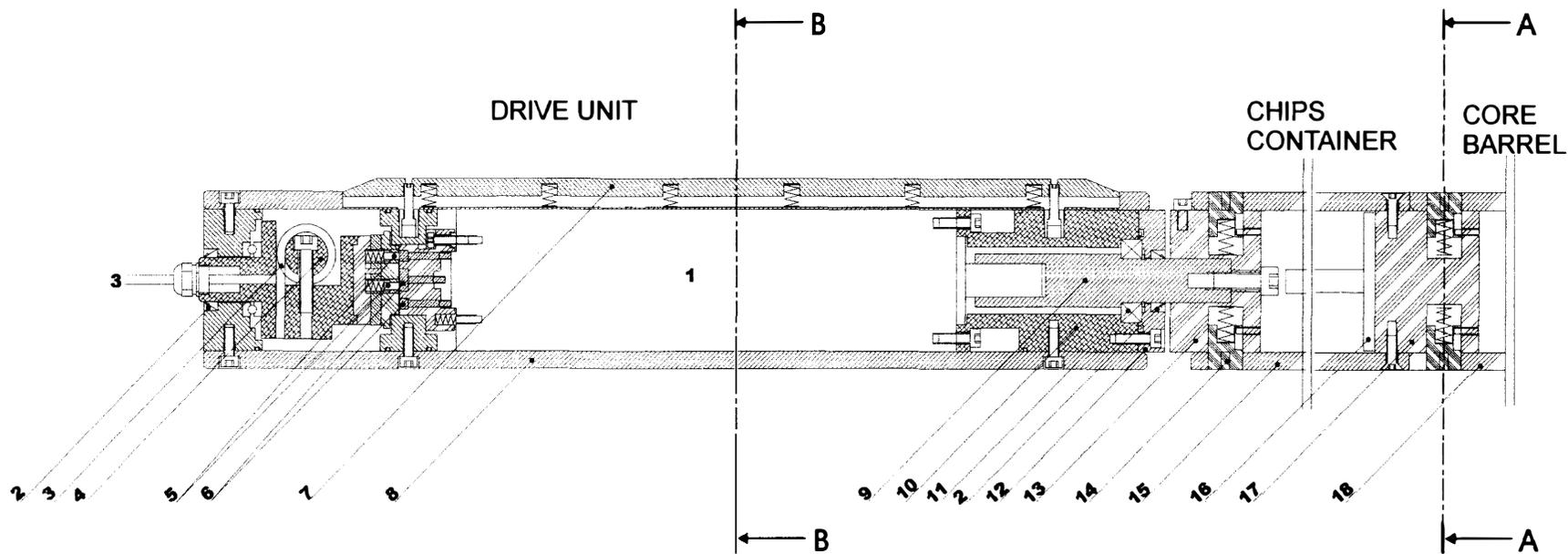
Fig. 4. Cross section design of the complete FELICS drill system. (1) DC-Motor (60 V, 4.2 A, Type Dunker GR 80×80) with reduction gear (Type PLG 70,  $r=28:1$ ), (2) circular seal (Lubroseal LM17C), (3) steel cable, (4) cable clamp, (5) electrical contactors, (6) slip-ring, (7) anti-torque system, (8) jacket, (9) shaft, (10) motor support, (11) ball bearing, (12) bearing cover, (13) motor clutch, (14) clutch bolt, (15) chips container, (16) chips extractor, (17) drill clutch, (18) core barrel.
