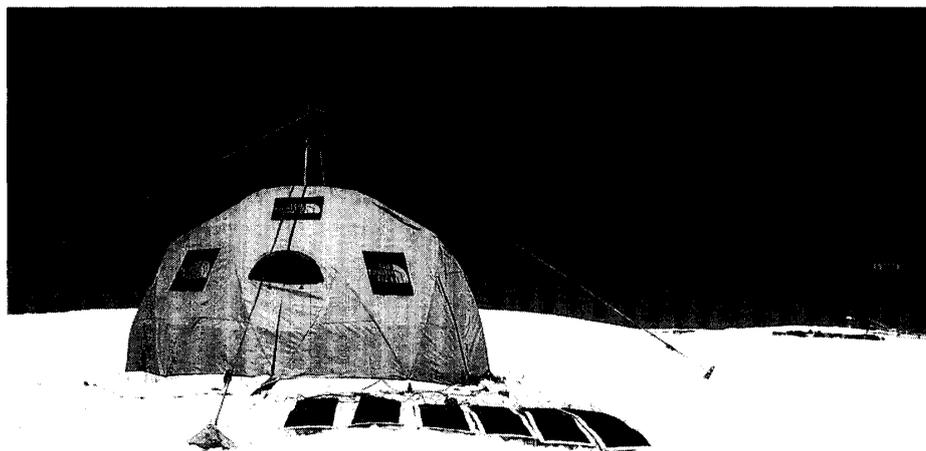
Fig. 1. Installation of FELICS inside the protective tent on top of Cerro Tapado (Chile, 5536 m a.s.l.) in February 1999. The 6 flexible solar panels used as a power supply are visible in the front.
