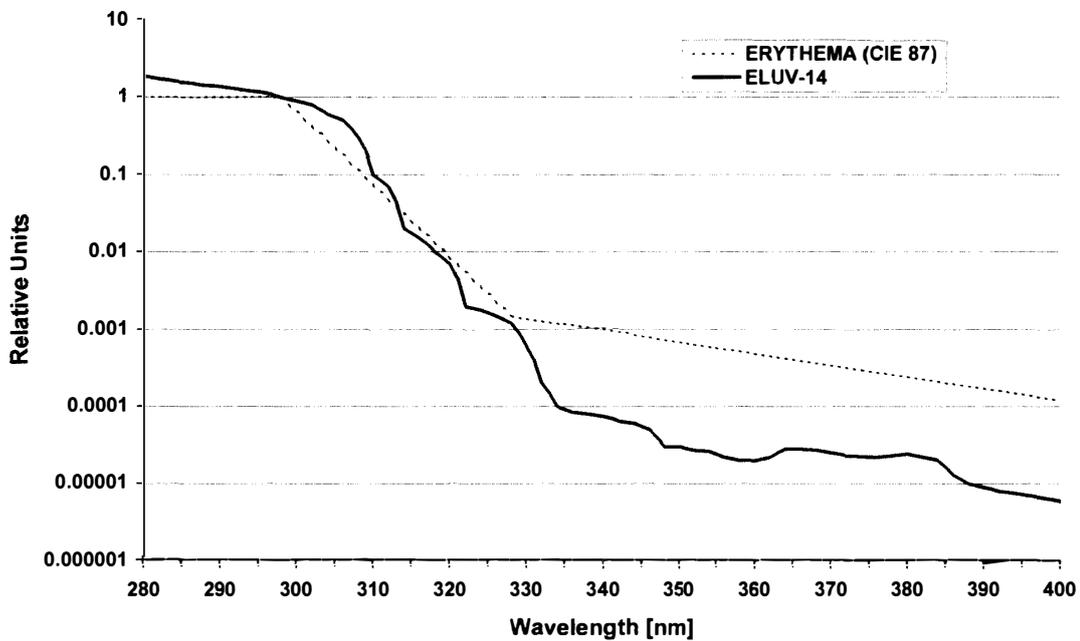
Fig. 2. Spectral sensitivity of the ELUV-14 dosimeter (solid line) and the standard erythemal spectra CIE 87 (dashed line).
