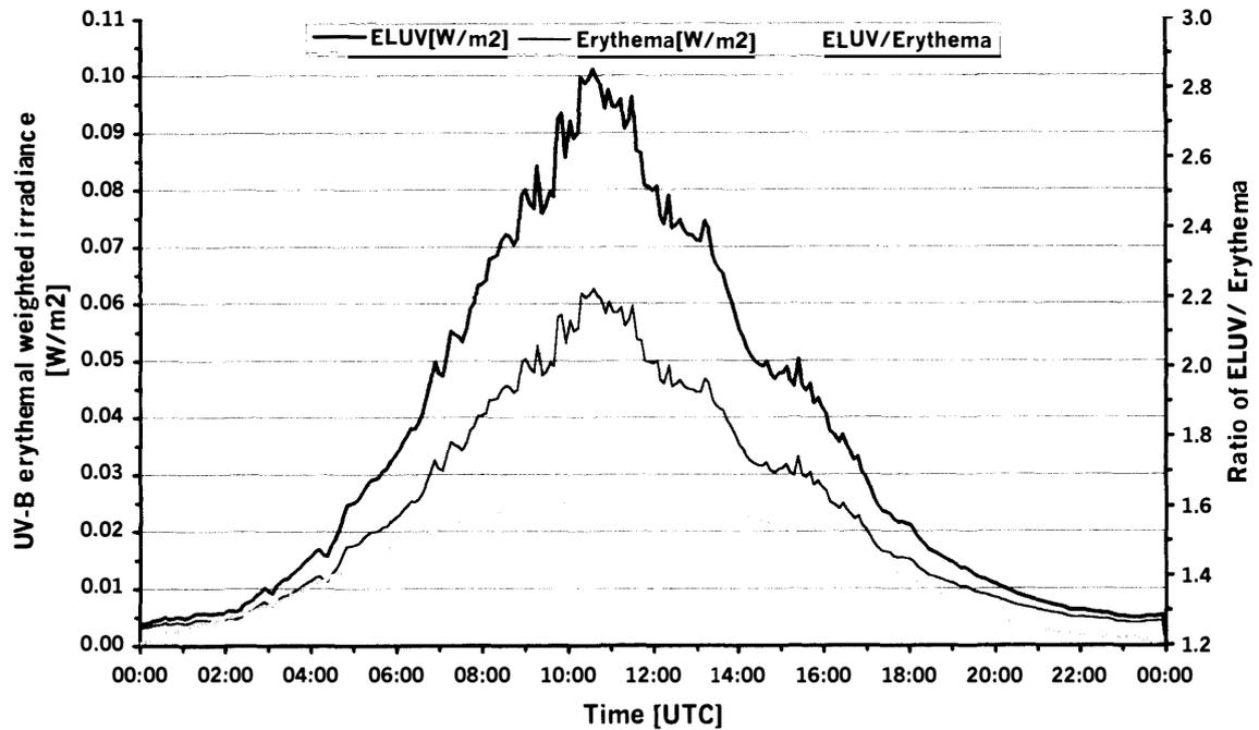
Fig. 3. Diurnal variation of ELUV-14 (bold line) and erythemal (thin line) weighted UV-B irradiances derived from spectral radiometer data recorded at Koldewey-Station on June 8, 1999. The ratio ELUV-14/Erythema (lower curve) is the transformation function between both weighted irradiances for this day.
