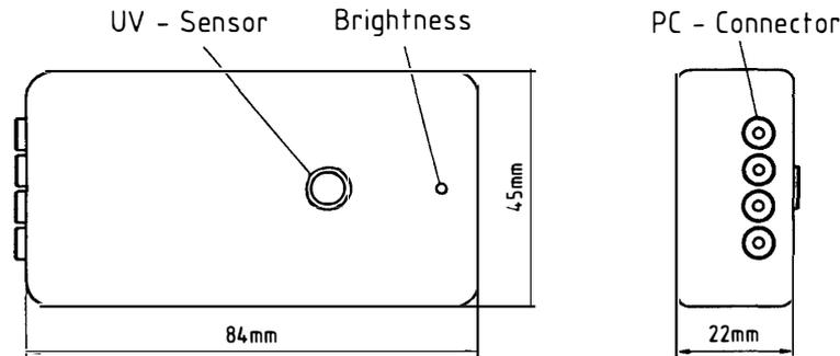
Fig. 1. A drawing of the ELUV-14 dosimeter illustrating size and position of sensors.
