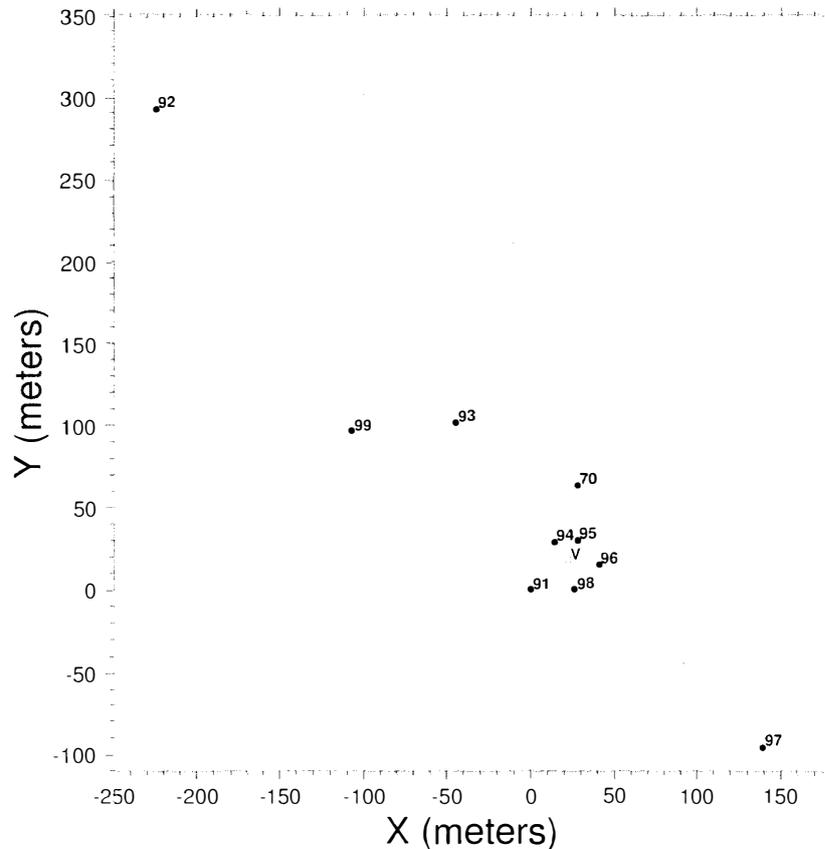
Fig. 5. The local control network around the Ny-Ålesund VLBI antenna. The VLBI antenna position (its azimuth axis) is marked by an open circle and a letter V. The pillars are marked with filled circle and the reference number used also in Table 1. The origin of the axis is pillar 91. The pillars 99 and 70 are not permanent and have been added using a tripod.
