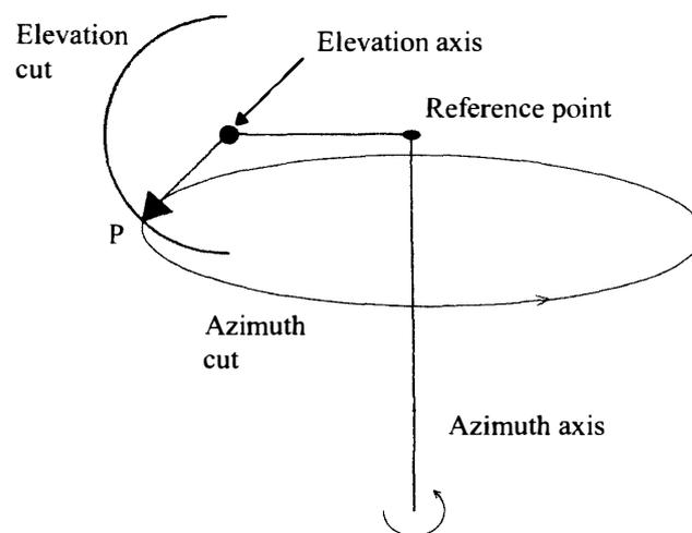
Fig. 2. A scheme of the motion of a generic point on the antenna during a rotation in azimuth and in elevation.
