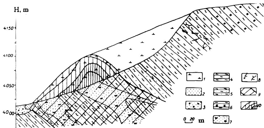
Fig. 1. The geochemical field above the ore zone and the endogenic halo. 1-ice; 2-sand; 3-gravel; 4-shale; 5-sandstone; 6-limestone; 7-ore body; 8-shatter zone; 9-endogenic halo; 10-geochemical field in the ice (spacing in cross-hatch shows the degree of contrast of the geochemical field).
