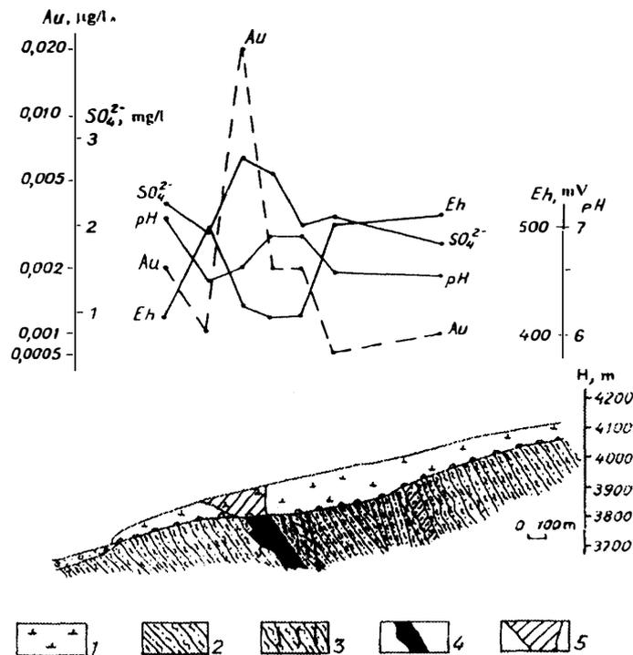
Fig. 4. Geochemical profile along the surface of Davidov Glacier above the ore zone.
