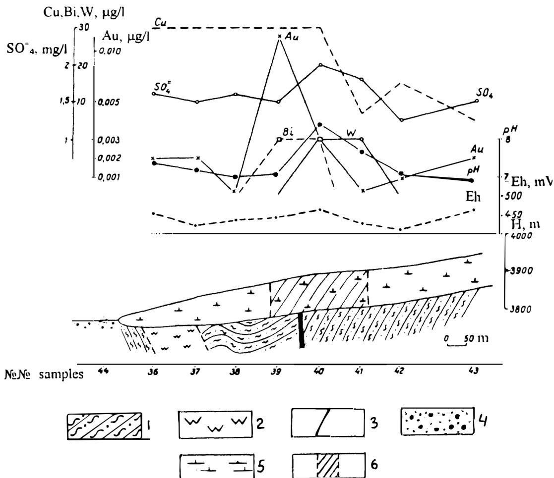
Fig. 3. Geochemical profile along the surface of Boordu Glacier above the ore zone. 1-metamorphic shale; 2-metasomatic rock; 3-ore metasomatite; 4-sandy shale; 5-glacier; 6-cryogenic halo.
