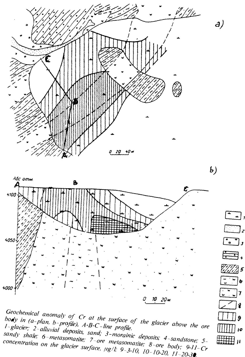
Fig. 2. Geochemical anomaly of Cr at the surface of the glacier above the ore body in (a-plan, b-profile), A-B-C-line profile.
