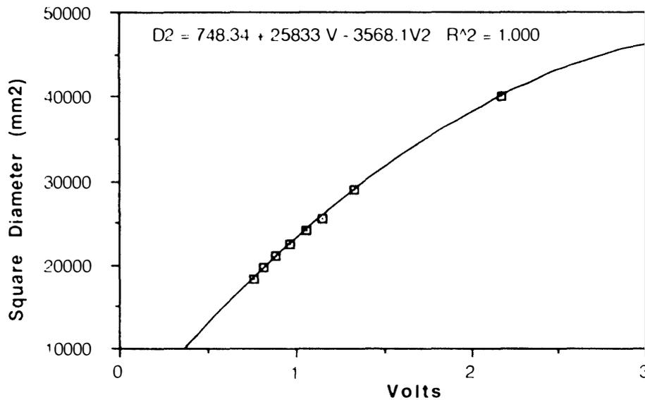
Fig. 5. Calibration curve obtained for the caliper.
