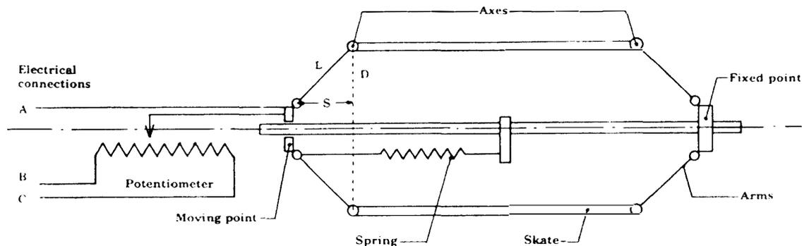
Fig. 4. Principle of the caliper. In the right triangle we can write:  $(D-D_0)^2=L^2-S^2$  ( $D_0$  and  $L$  are constants). For the linear potentiometer the voltage between ends A and B is:  $V_{AB}=aS+b$  ( $a$  and  $b$  are constants). As  $D_0$  is small, the equation of the caliper can be written  $D^2=a'+b'V_{AB}-c'V_{AB}^2$  ( $a'$ ,  $b'$ ,  $c'$  are parameters adjusted from the calibration).
