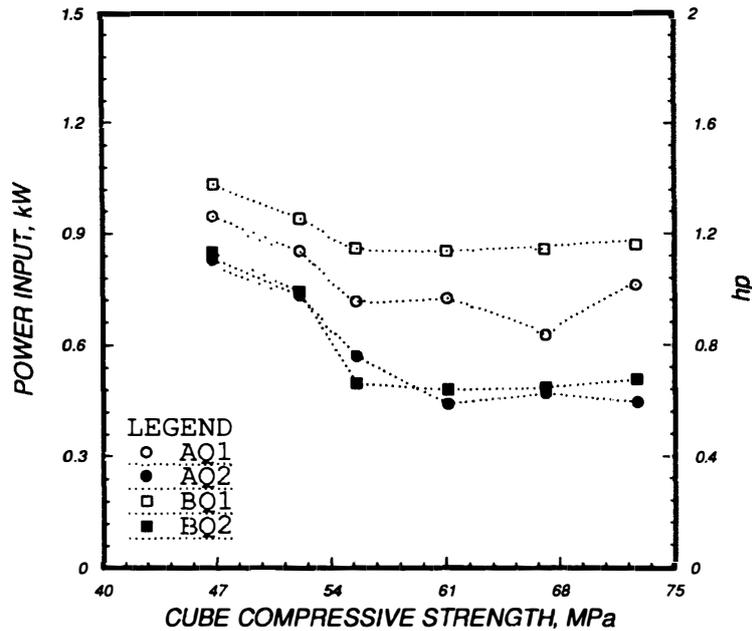
Fig. 8. Power consumption vs. cube compressive strength of rock.
