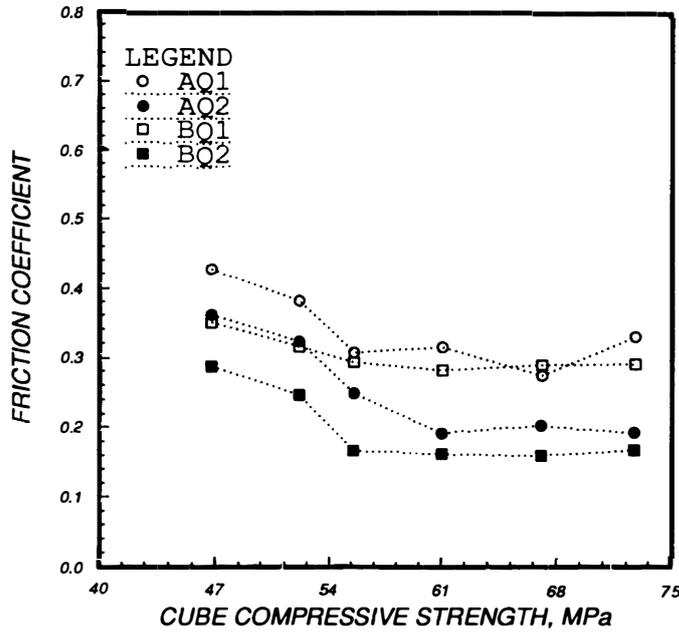
Fig. 10. Friction coefficient vs. cube compressive of rock.
