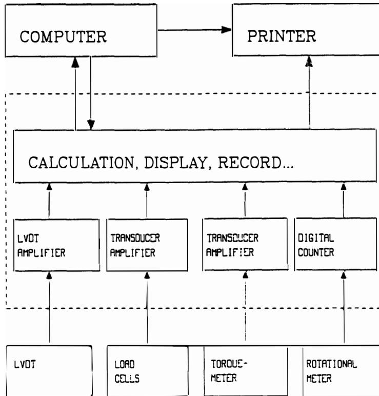
Fig. 4. Flow chart of laboratory testing procedures.
