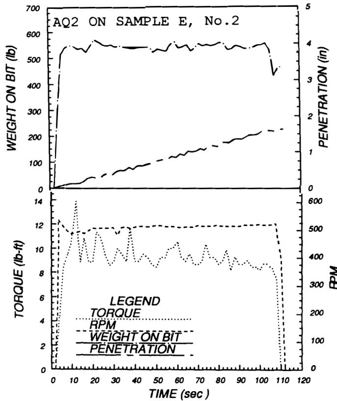
Fig. 5. An example of original data from laboratory drilling test.
