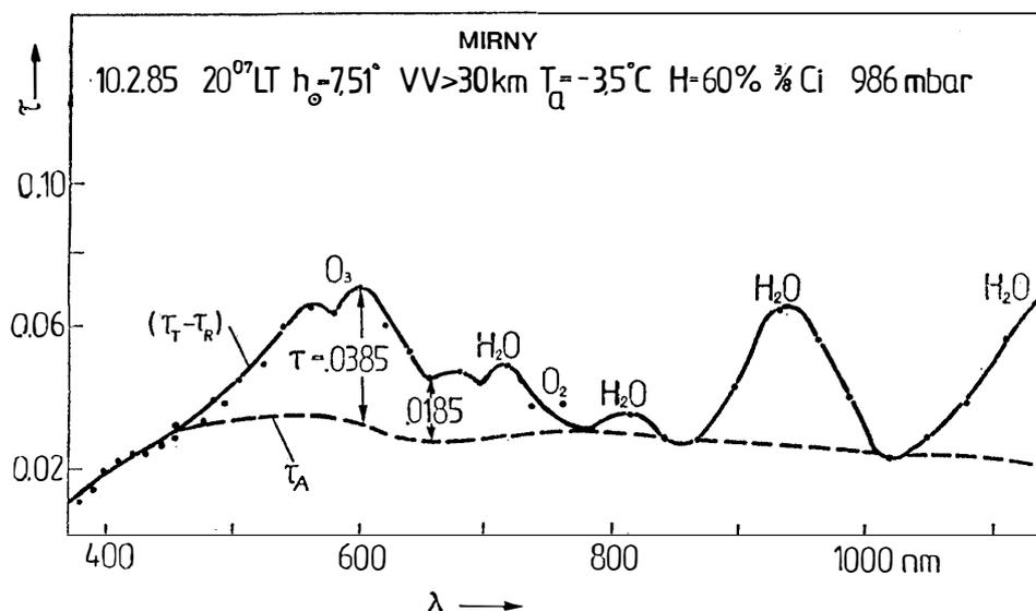
Fig. 1. Diagram showing the graphical smoothing of the  $(\tau_T - \tau_R)$ -curve to eliminate the optical thickness of water vapour, ozone and oxygen. *VV*: visibility,  $T_a$ : air temperature, *H*: relative humidity, *Ci*: Cirrus clouds.
