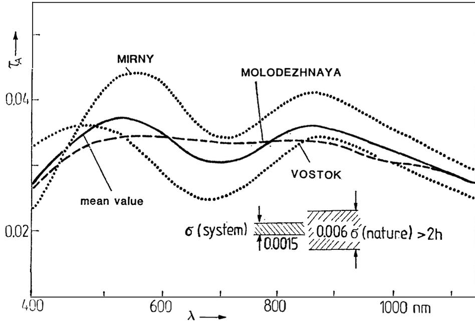
Fig. 2. Mean values of the aerosol optical thickness  $\tau_A$  at 3 Antarctic stations, Molodezhnaya, Vostok, Mirny in the summer of 1984/85.
