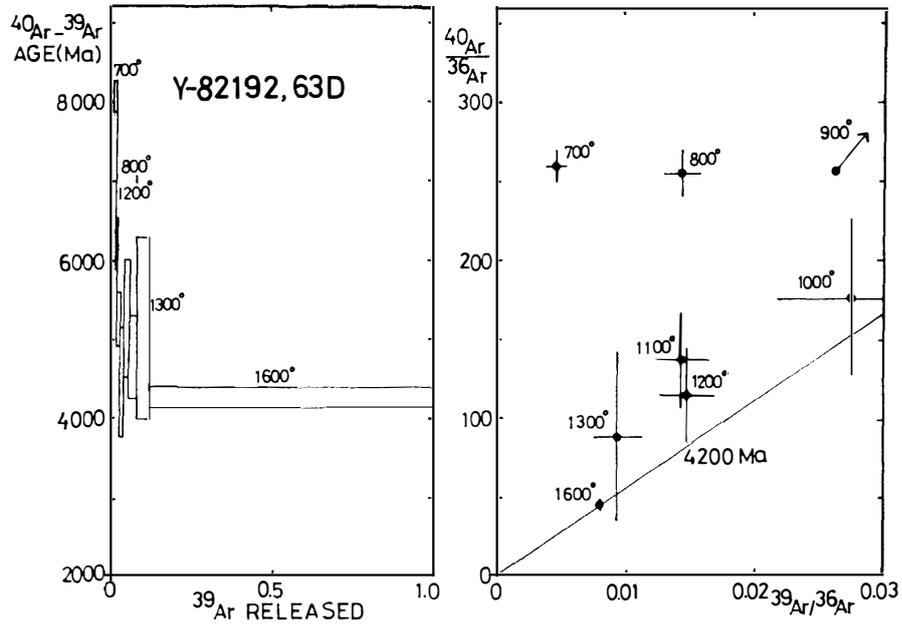
Fig. 1. The  $^{40}\text{Ar}$ - $^{39}\text{Ar}$  age diagram and the  $^{40}\text{Ar}/^{36}\text{Ar}$ - $^{39}\text{Ar}/^{36}\text{Ar}$  plot for the sample Y-82192,63D (clast+matrix). The number at each column indicates the degassing temperature in degree Celsius. The uncertainty is indicated by  $1\sigma$ . In the  $^{40}\text{Ar}/^{36}\text{Ar}$ - $^{39}\text{Ar}/^{36}\text{Ar}$  plot, a reference isochron of 4200 Ma is shown.
