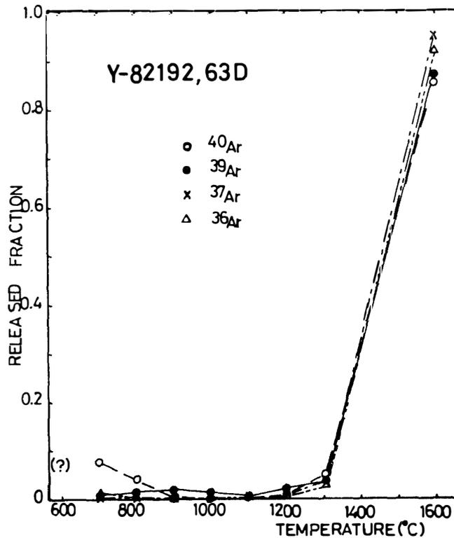
Fig. 2. The release patterns of Ar isotopes for Y-82192,63D. Note that most Ar is degassed in the highest temperature fraction.
