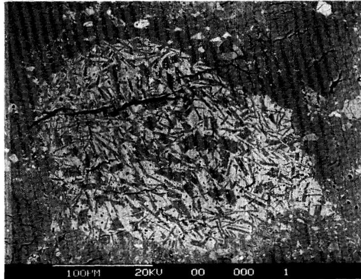
c. Fine-grained impact melt breccia with a subophitic to variolitic texture from Y-82192.
