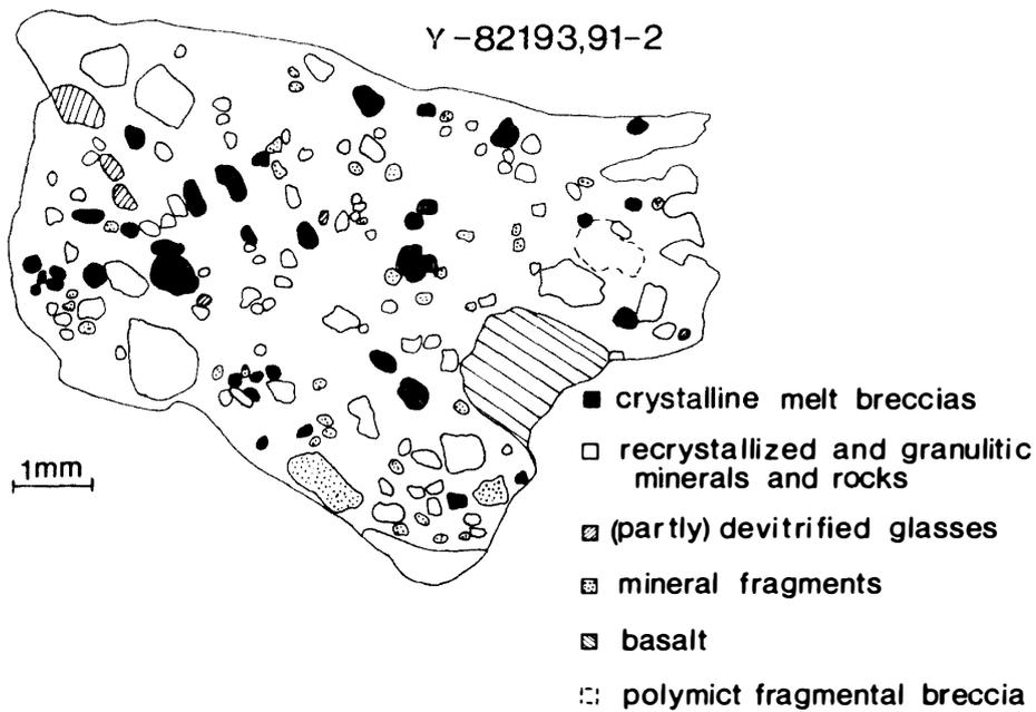
Fig. 2. Sketch map of thin section Y-82193,91-2 showing the distribution of mineral and lithic clasts.
