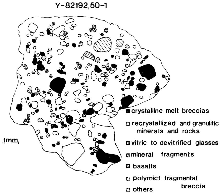
Fig. 1. Sketch map of thin section Y-82192,50-1 showing the distribution of mineral and lithic clasts.
