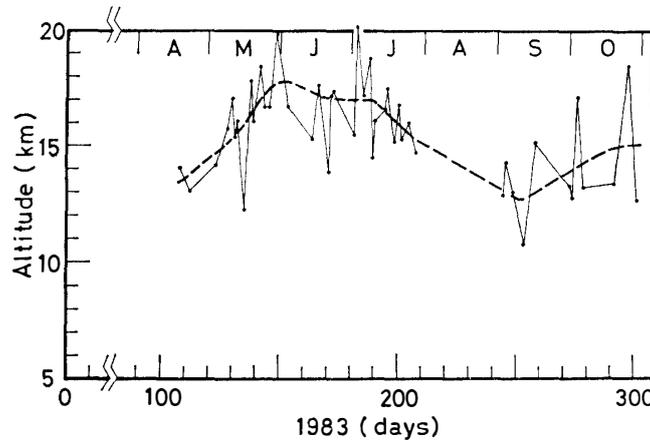
Fig. 1. The height of aerosol layer ( $h_B$ ) defined by  $\int Z \beta(Z) dZ / \int \beta(Z) dZ$ ,  $\beta(Z)$  is aerosol backscattering coefficient. This value gradually decreased after early July.
