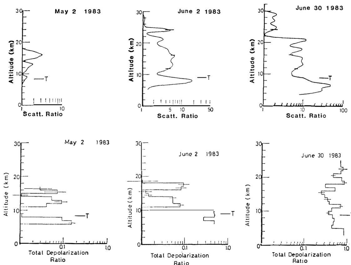
Fig. 4. Typical measurements of scattering ratio and depolarization ratio at Syowa Station. The measurements on May 2, June 2, and June 30, 1983 show the typical feature of pre-enhancement stage, early enhancement, and fully developed enhancement, respectively.
