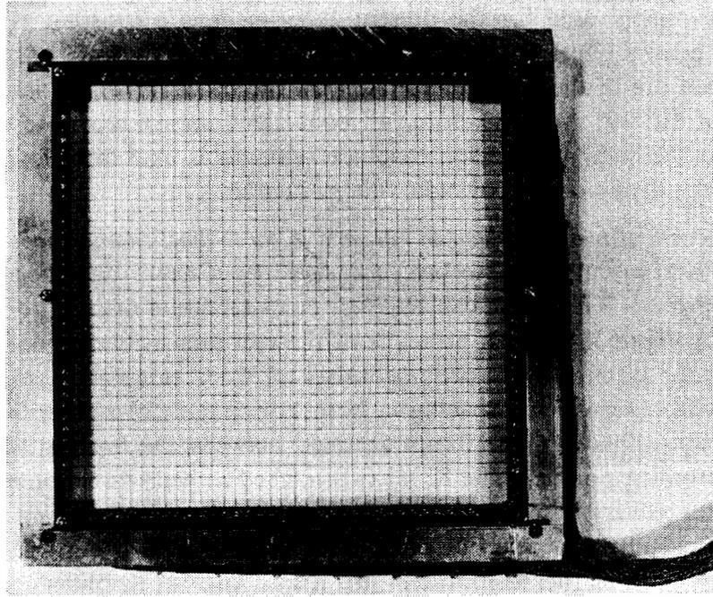
*Fig. 5. Proto-type of two-dimensional current probe. 32 tungsten wires (0.15 mm in diameter) are stretched in horizontal and vertical directions, respectively. The spacings between the parallel wires are 5 mm. They are connected to multiplexers for the respective directions. The effective measurement area is  $15.5 \times 15.5$  cm<sup>2</sup>. The effective transparency of the two-dimensional probe is 94%.*
