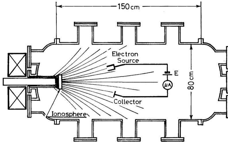
Fig. 2. *Experimental setup. Electron source, collector and model ionosphere are arranged in a horizontal plane which includes the main axis of the magnetic field. The gas pressure in the chamber is order of  $10^{-6}$  Torr.*
