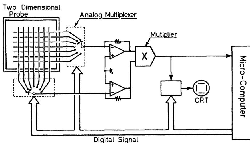
Fig. 4. Principle of two-dimensional current probe and data acquisition system. The horizontal and vertical wires are held 2 mm apart from each other. In the CRT, two-dimensional distribution of beam currents is displayed on real-time basis.
