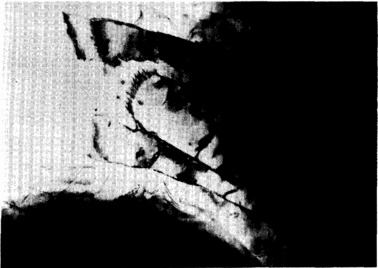
b. Subgrain boundaries and tilt boundaries. Bright field image. Width 7.5 \mu\text{m} .
