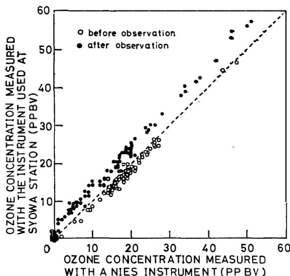
Fig. 1. Calibration of the Dasibi ozone meter used at Syowa Station with the one at the National Institute for Environmental Studies.
