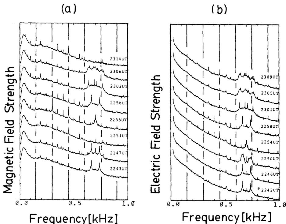
Fig. 5. The magnetic (a) and the electric (b) field spectra from 40 Hz to 1 kHz observed on the balloon  $B_{15}$ -2N around the start time of a geomagnetic substorm. Time of the spectrum advances from the bottom to the top. It should be noted that the spectral enhancement from 620 to 800 Hz is caused by the interference from the other instrument on board the balloon  $B_{15}$ -2N. The positions of harmonic frequencies of 150 Hz are indicated by the vertical lines.
