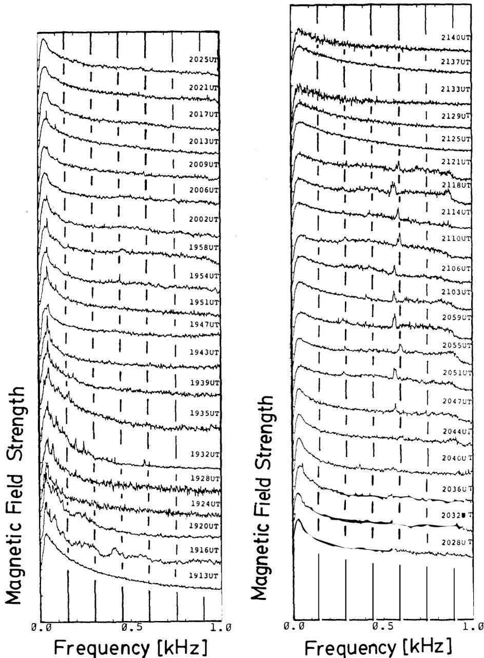
Fig. 3. Magnetic field spectra from 40 Hz to 1 kHz observed on the balloon  $B_{15-1N}$ . Time of the spectrum advances from the lower-left to the upper-right. The positions of harmonic frequencies of 150 Hz (150, 300, 450, 600 and 750 Hz) are indicated by the vertical lines.
