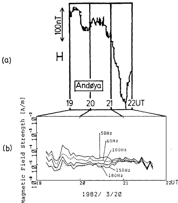
Fig. 2. Strength variations of power line radiations observed by the balloon  $B_{15-1N}$  versus geomagnetic field variations.
