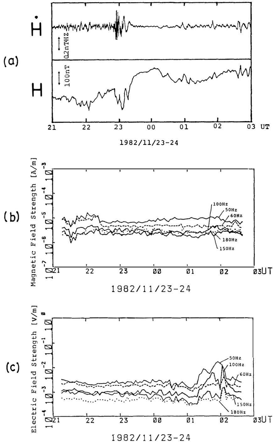
Fig. 4. Strength variations of power line radiations observed on the balloon  $B_{15-2N}$  and their relation to geomagnetic field variations.
