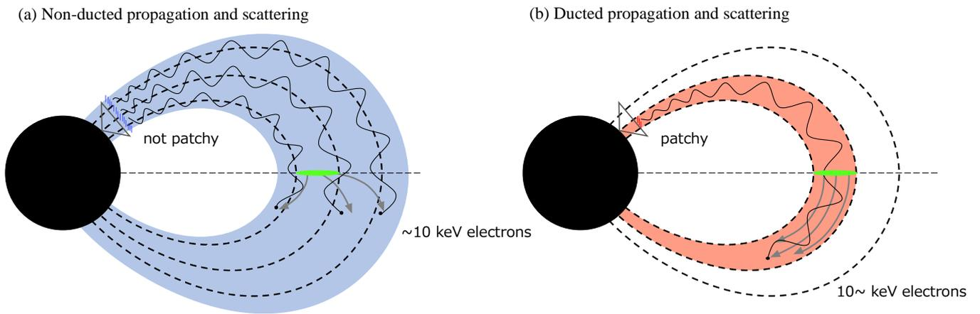
Figure 1. Schematic diagram showing the relationship between pulsating aurora, ducts, and chorus wave propagation. (a): In the case of non-ducted propagation and scattering, resonance energy is low and PsA structure is not patchy. (b): In the case of ducted propagation and scattering, resonance energy is high and PsA structure is patchy.
