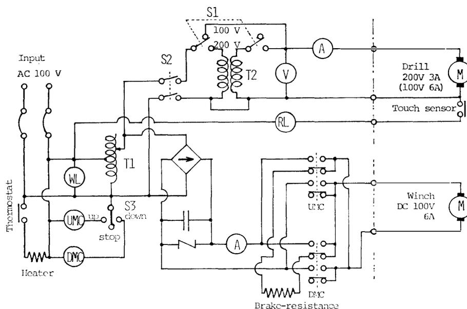
Fig. 2. Circuit diagram of C251.
