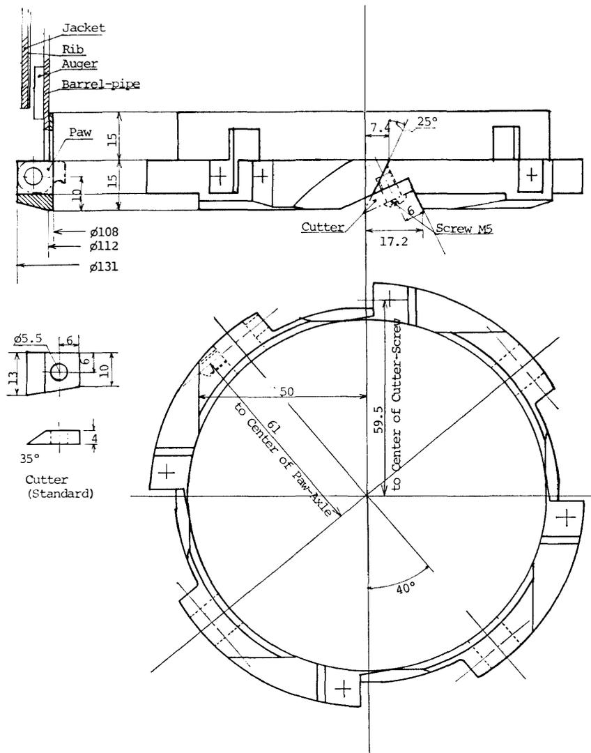
Fig. 1. Cutter holder of B251 and standard cutter. (A short paw is shown in the figure. A long paw is oppositely placed.)
