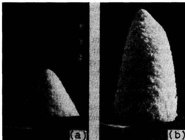
Fig. 2. A cone-shaped deposit for the measurement of the repose angle: (a) in the case of no precipitation and (b) in the case of snow falling.
