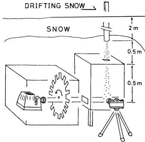
Fig. 3. Measurement system for fall velocity of drifting snow particles.
