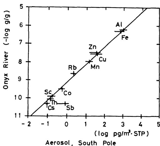
Fig. 5. Relationship of trace element contents between the Onyx River water and the South Pole aerosol particle (data of aerosols are from MAENHAUT *et al.*, 1979).
