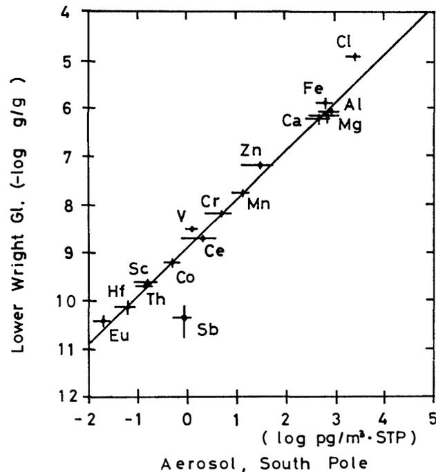
Fig. 10. Relationship of trace element contents between the Lower Wright Glacier ice and the South Pole aerosol particle.
