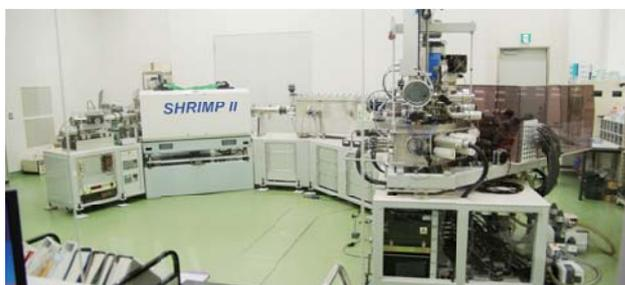
Sensitive high resolution ion microprobe (SHRIMP) for age dating of minerals.
