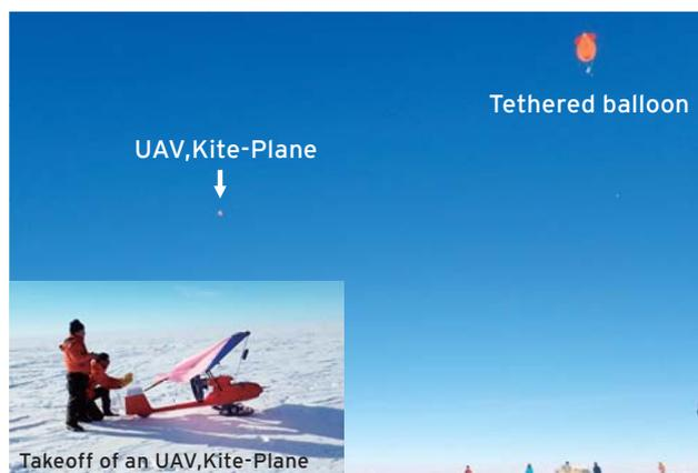
Atmospheric observation above the Antarctic ice sheet with unmanned aerial vehicle (UAV) and tethered balloon
