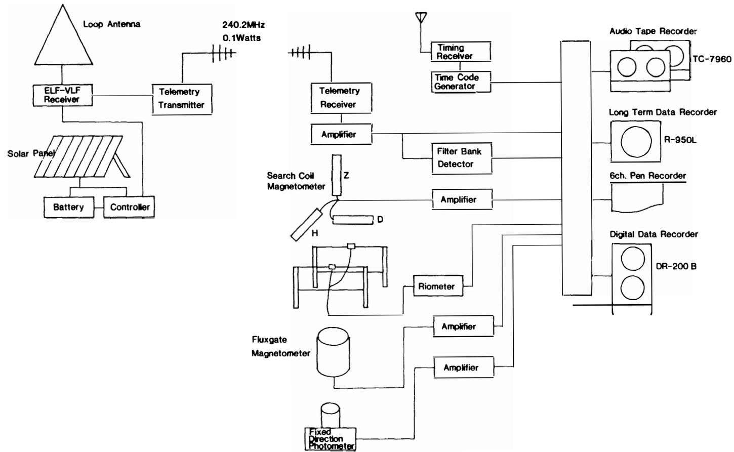
Fig. 4. Block diagram of the observation system installed at Isafjördur and Husavik.
