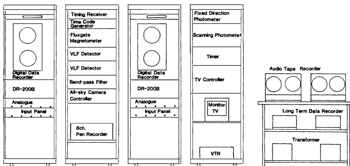
Fig. 3. A layout of the observation system at Husafell.
