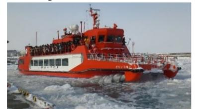
Fig. 6 Sightseeing icebreaker Garinko II with Archimedes' screws
