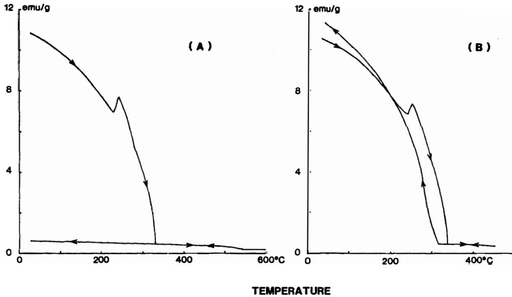
Fig. 12. Thermomagnetic curves of natural pyrrhotite grains (magnetic field = 10 kOe). (A) Heated up to 660°C. (B) Heated up to 480°C.
