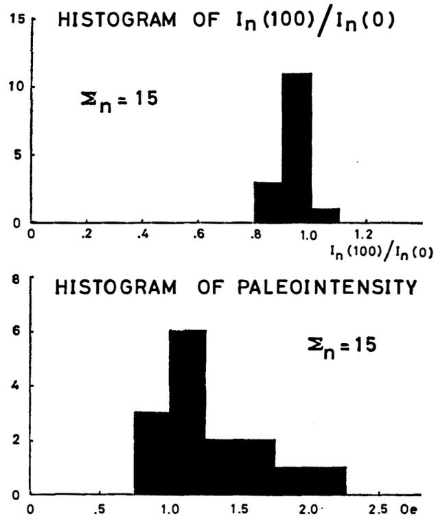
Fig. 6. (Top) Histogram of ratios of residual NRM intensity ( $I_n(100)$ ) after AF-demagnetizing to 100 Oe peak to initial NRM intensity ( $I_n(0)$ ) for 15 chips of the Allende bulk rock. (Bottom) Histogram of paleointensities for 15 chips of the Allende bulk rock.
