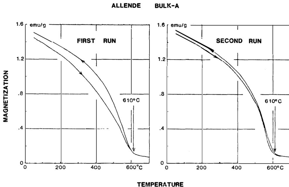
Fig. 2. Thermomagnetic curves of a bulk specimen (A) of the Allende, first-run and second-run curves (magnetic field = 10 kOe).
