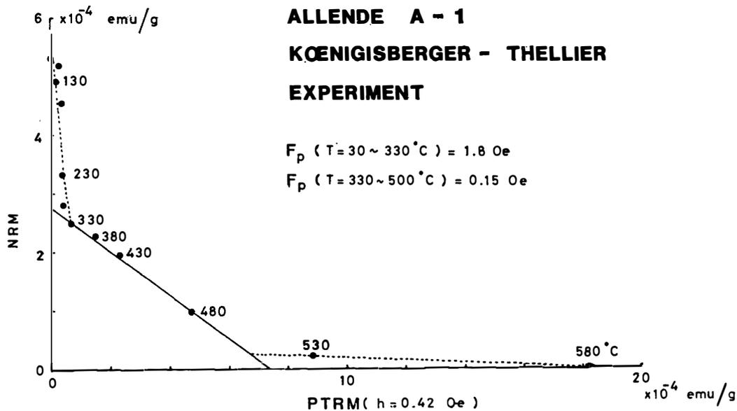
Fig. A-3. Königisberger-Thellier plots for an Allende bulk specimen including small fragments of fusion crust.
