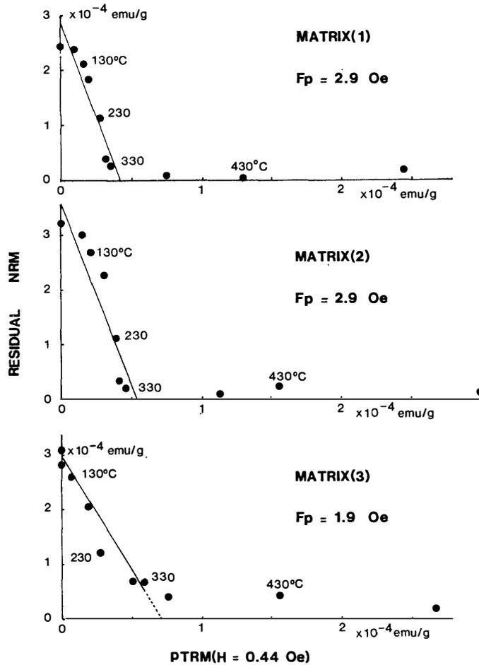
Fig. 18. Königisberger-Thellier plots for 3 Allende matrix specimens (magnetic field for acquisition of PTRM=0.44 Oe).
