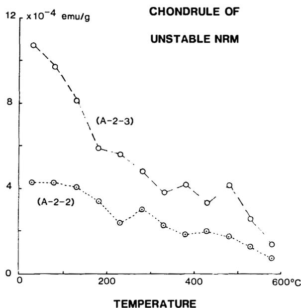
Fig. 11. Thermal demagnetization curves of NRM intensity for 2 Allende chondrules which have unstable NRM.
