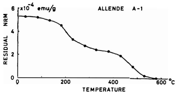
Fig. A-2. Thermal demagnetization curves of NRM of Allende bulk specimen including small fragments of fusion crust. (Top) Projection of residual NRM vectors on (X-Y) and (Y-Z) planes. (Bottom) Thermal demagnetization curve of NRM intensity.
