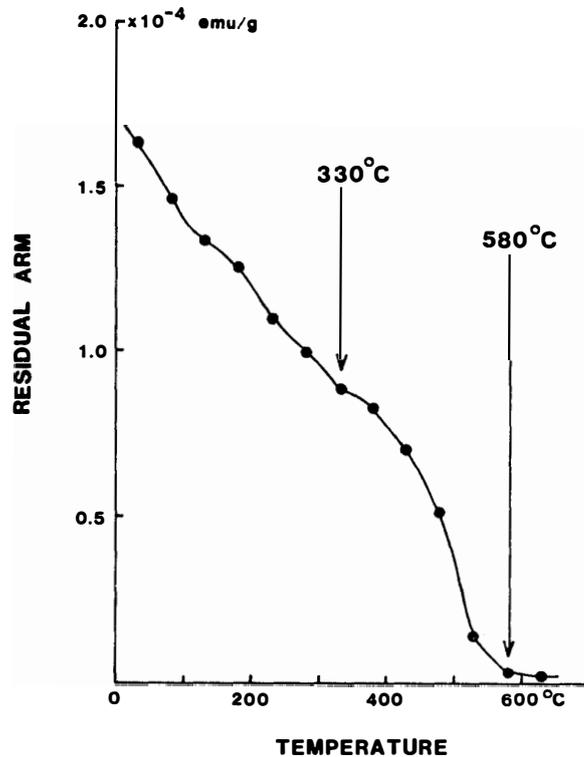
Fig. 13. Thermal demagnetization curve of ARM intensity of bulk specimen of the Allende (C3). ARM is acquired in  $\bar{H} = 1400$  Oe peak in applied alternating magnetic field and in  $h = 0.44$  Oe in coaxially applied steady magnetic field.
