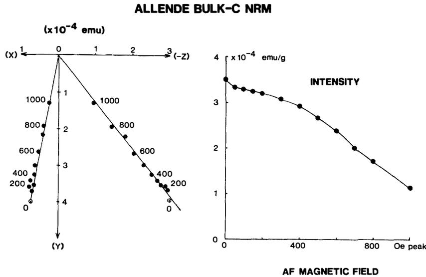
Fig. 4. AF-demagnetization curves of NRM of a bulk specimen (C) of the Allende. (Numeral figures for plots in the left diagram are AF-demagnetizing fields in unit of Oe peak.)
