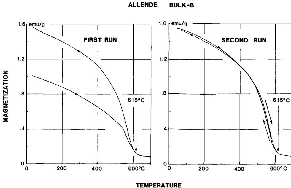
Fig. 3. Thermomagnetic curves of a bulk specimen (B) of the Allende, first-run and second-run curves (magnetic field = 10 kOe).
