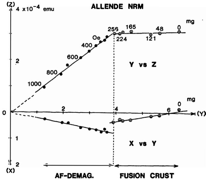
Fig. A-1. Changes of residual NRM caused by successively scraping off fusion crust layer (right half) and changes of residual NRM of uncontaminated interior by AF-demagnetization (left half) of an Allende bulk sample with a fusion crust layer, projected on (X-Y) and (Y-Z) planes.
