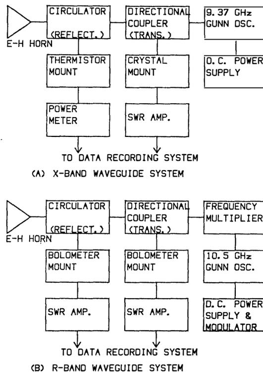
Fig. 1. Block diagrams of the experimental apparatus.
