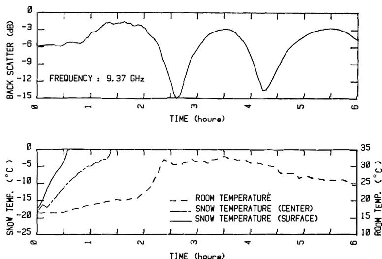
Fig. 5. Variations of the intensity of back scatter of 9.37 GHz wave and the room and snow temperatures against the time.
