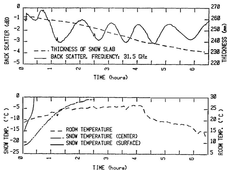
Fig. 7. Relations between the thickness of snow slab and the periodic fluctuation of the back scatter at the frequency of 31.5 GHz.
