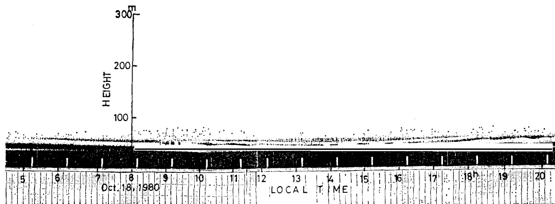
Fig. 5. Acoustic sounder's facsimile record during stable stratification. Period: 0500 LT to 2000 LT, October 18, 1980.
