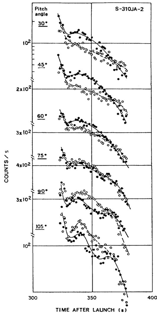
Fig. 3. A part of intensity-time profiles of particles measured by the proportional counter aboard the S-310JA-2 rocket. Solid and open circles correspond to the two spin phases in which the pitch angles are increasing and decreasing, respectively.
