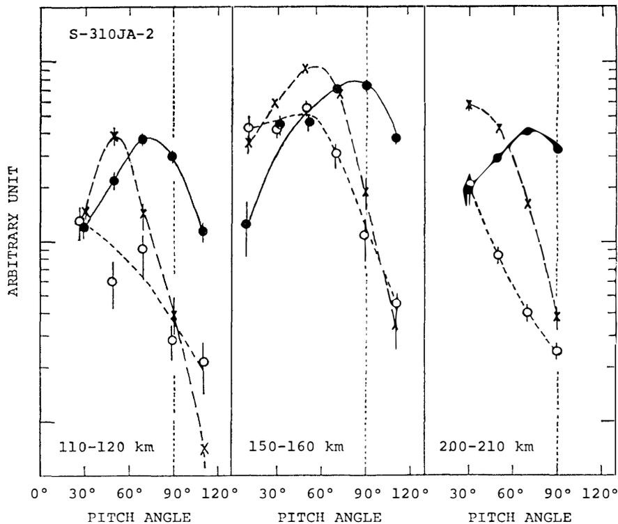
Fig. 4. Pitch angle distributions of particles during the descending phase of the S-310JA-2 rocket flight. Solid and open circles mean the proportional and scintillation counters magnetically shielded using permanent magnet, respectively. Cross marks are for the non-shielded scintillation counter. The respective rocket altitudes at which the pitch angle distributions were deduced are shown in the lower portion of diagram.
