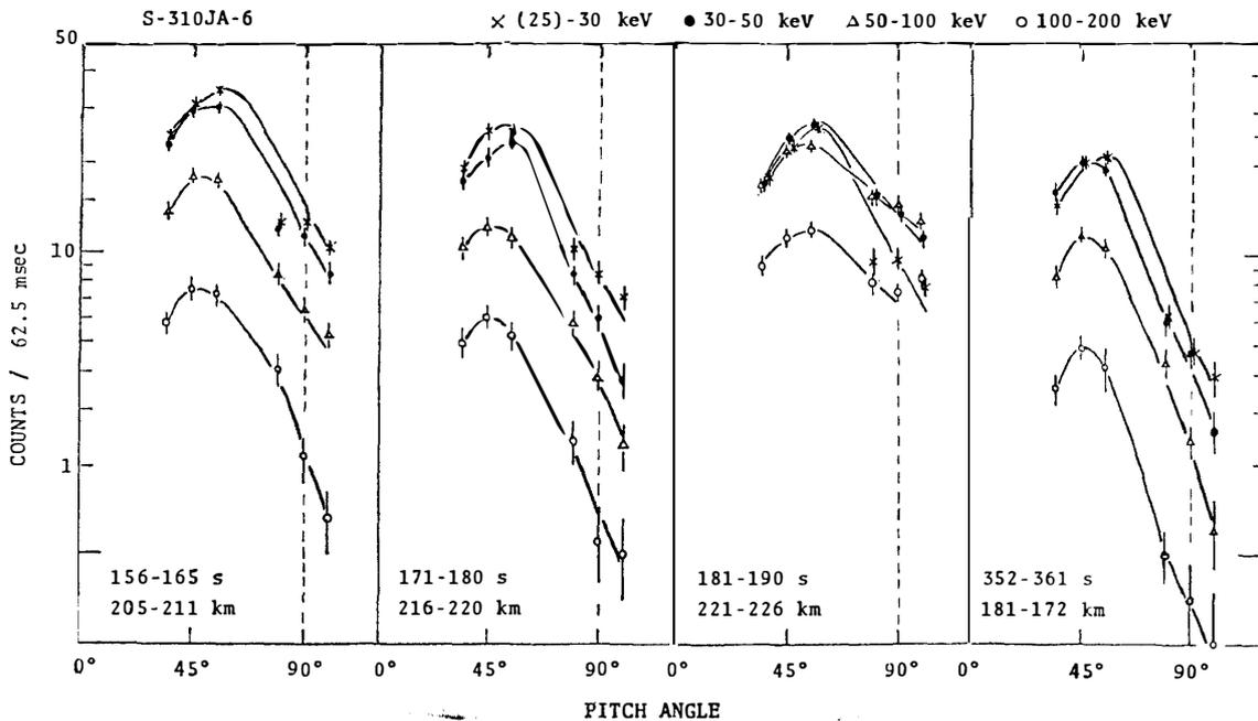
Fig. 6. Pitch angle distributions of particles measured by the proportional counter aboard the S-310JA-6 rocket. They refer to four energy channels and four time intervals.
