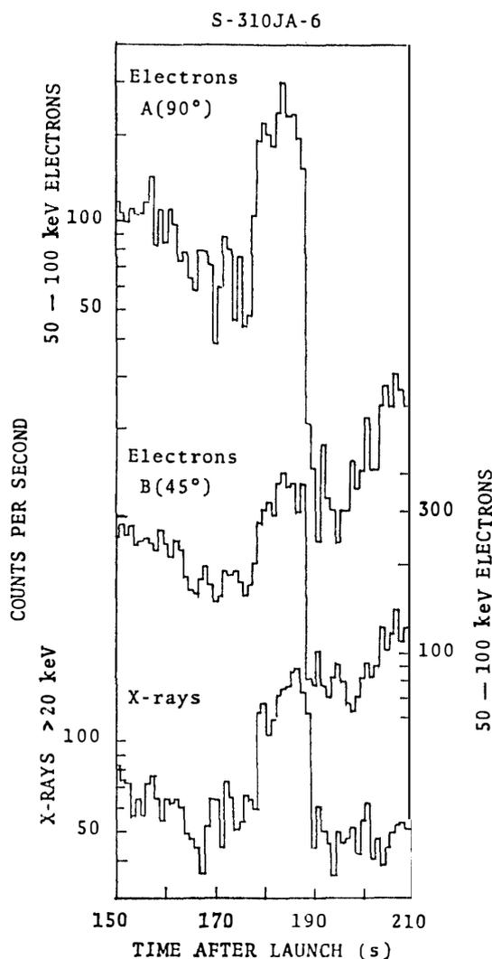
Fig. 5. A part of time variations of particle intensities measured in the S-310JA-6 rocket experiment. Upper and middle curves are those from the proportional counters mounted making angles  $90^\circ$  and  $45^\circ$  against the rocket axis, and the lower is for X-rays.
