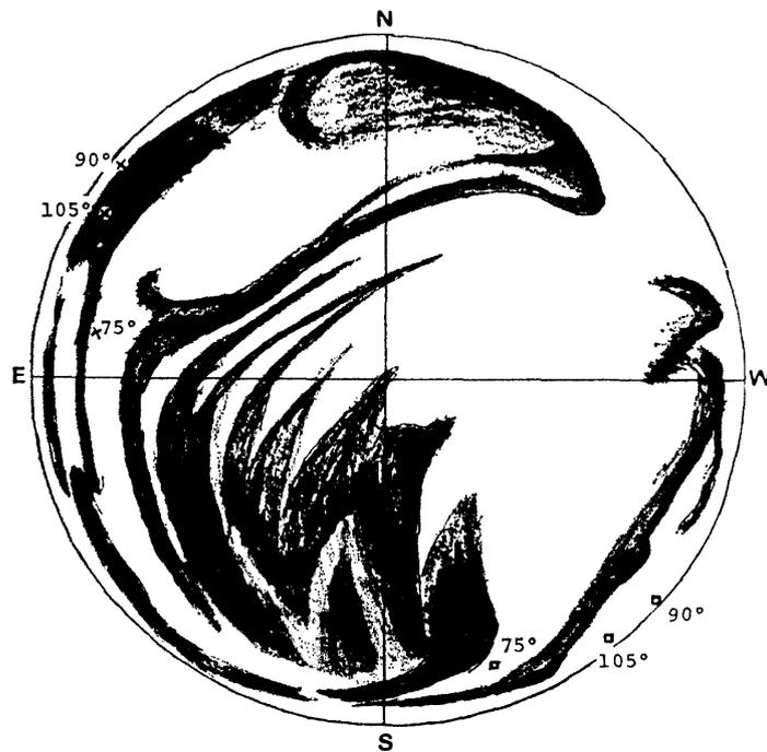
Fig. 8. A relation between the viewing directions of the rocket-borne particle detector and the locations of auroral visual arcs. The viewing directions corresponding to the two different spin phases with a selected pitch angle of  $75^\circ$ ,  $90^\circ$  or  $105^\circ$  are plotted on the auroral arc pattern, indicated by black area, reproduced from all-sky camera photograph.
