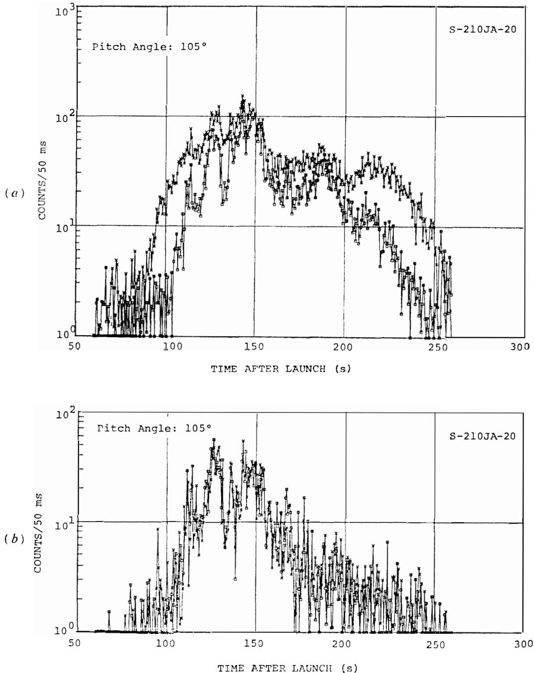
Fig. 2. Intensity-time profiles of particles measured in the S-210JA-20 rocket experiment. Particle fluxes are given for the two different spin phases with the same pitch angle of  $105^\circ$ . Two symbols, cross and square, represent the two spin phases in which the pitch angles are increasing and decreasing, respectively. a) For the proportional counter, and b) for the scintillation counter.
