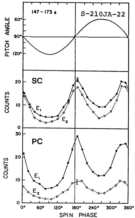
Fig. 1. Changes of the pitch angle and the particle counts from SC (scintillation counter) and PC (proportional counter) during a spin. A time interval from 147 s to 173 s after launch is sampled in the case of the S-210JA-22 rocket.  $E_1$  and  $E_2$  correspond to the different energy channels.
