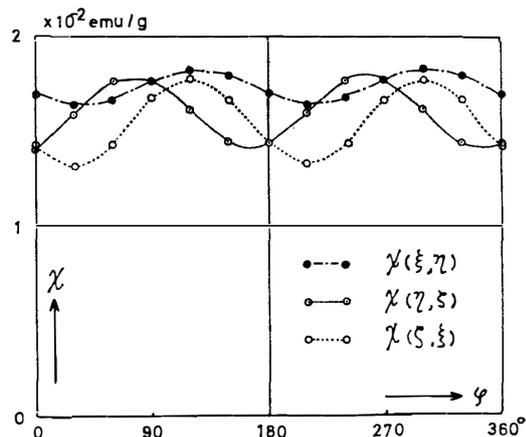
Fig. 6. Magnetic susceptibility anisotropy curves for Mt. Baldr b chondrite.
