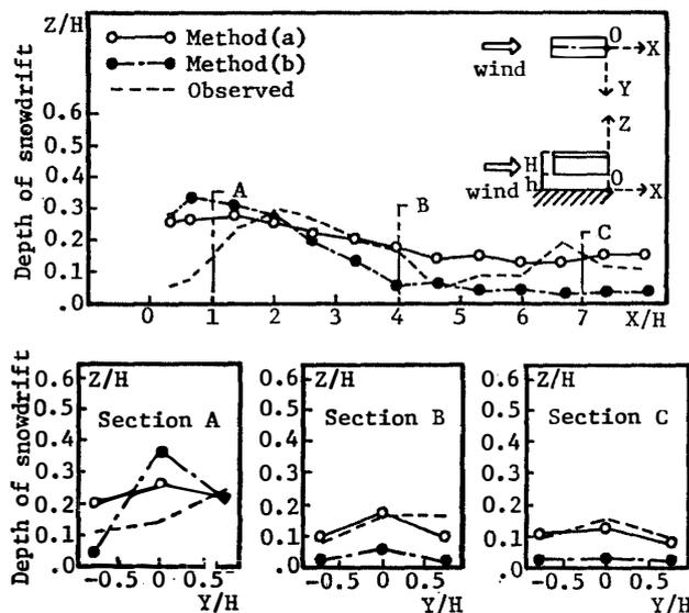
Fig. 6. Comparison of wind tunnel experiments and observations for the Observation Hut. Observations were in April 1978.
