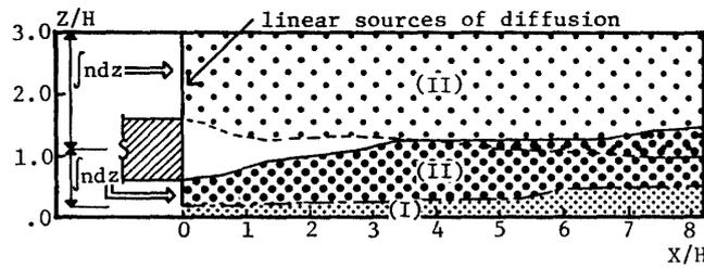
Fig. 5. Classification of the domain for drift density profile at the lee of the floor-elevated building.
