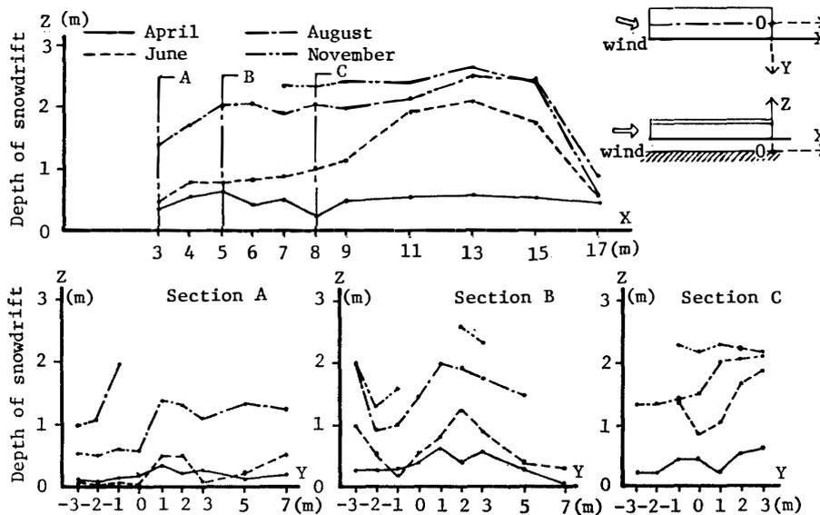
Fig. 4. Development of snowdrift in the lee of the Ionosphere Hut.
