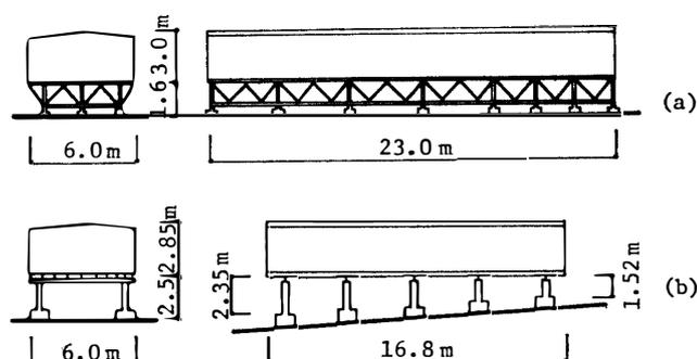
Fig. 2. Elevation of the buildings. (a) Observation Hut, (b) Ionosphere Hut.
