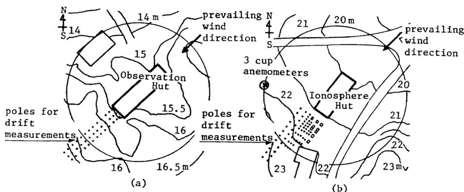
Fig. 1. Measurement area for drifted snow around the Observation Hut (a) and Ionosphere Hut (b) at Syowa Station.
