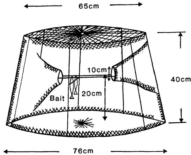
Fig. 2 Size and structure of the trap nets used in this study.
