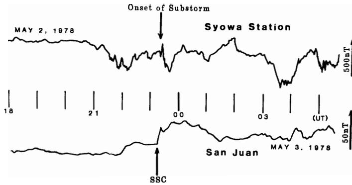
Fig. 5a. Ssc triggered substorm observed at Syowa on May 2, 1978 and the simultaneous H-component magnetogram at the middle latitude station, San Juan.
