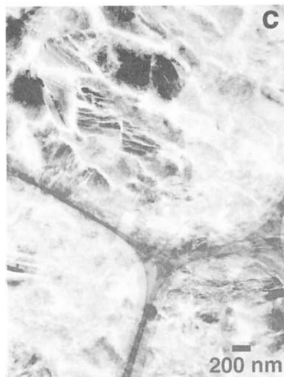
Figure 2 (a) A bright-field image of MM1. Incompletely dehydrated serpentine crystals show lamellar texture. (b) An enlarged image of a dehydrated serpentine crystal. (c) A low-magnification bright-field image of MM2. The matrix of MM2 is composed of coarse-grained serpentine (cronstedtite) and embedding very-fine grained material. A honeycomb network in this figure is a holey plastic supporting film.
