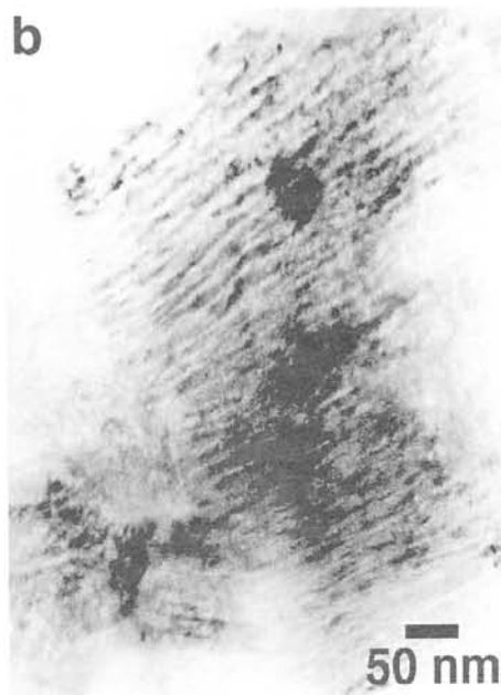
Figure 2 (a) A bright-field image of MM1. Incompletely dehydrated serpentine crystals show lamellar texture. (b) An enlarged image of a dehydrated serpentine crystal. (c) A low-magnification bright-field image of MM2. The matrix of MM2 is composed of coarse-grained serpentine (cronstedtite) and embedding very-fine grained material. A honeycomb network in this figure is a holey plastic supporting film.
