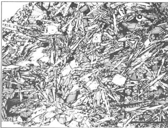
Fig. 1. Photomicrograph of the Sahara 99555 thin section (plane-polarized light). The section shows an ophitic texture mainly composed of lath anorthite with chemically zoned fassaite and Ca-rich olivine. Scale bar is 1 mm.
