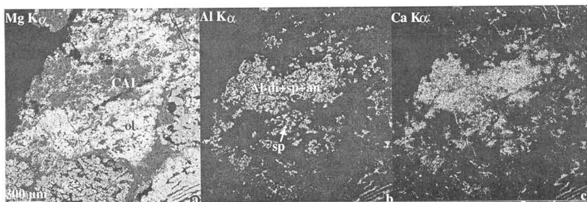
Fig. 3. X-ray elemental maps in Mg (a), Al (b) and Ca K \alpha (c) of an amoeboid olivine aggregate from Efremovka. The aggregate consists of forsteritic olivine (ol) and contains abundant CAIs composed of anorthite (an), Al-diopside (Al-di) and spinel (sp).
