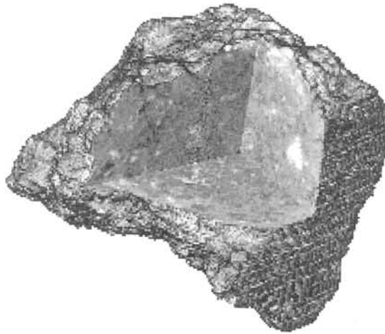
Figure 1. Three-dimensional structure of the Kobe meteorite C-5-1 (7-9 mm in size). Objects with bright, gray and dark contrasts are opaque minerals (pentlandite and magnetite), ferromagnesian silicates (olivine and pyroxene) and plagioclase, respectively.
