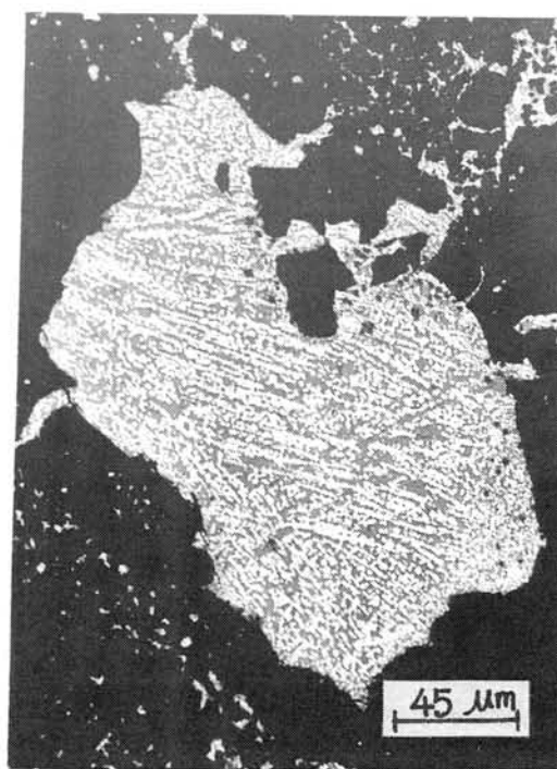
Fig.2 A metal-troilite eutectic nodule with very metal dendrites in a shock vein of Sixiangkou
