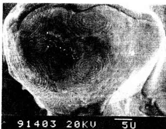
Fig.7 SEM image showing the well developed tetra-concentric-ring growth pattern on the tip of a elongated FeNi crystallite.
