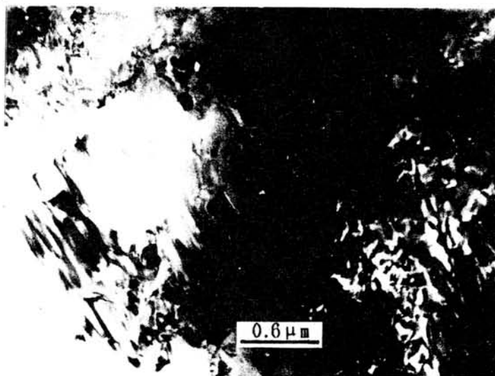
Photo 3 TEM image showing ringwoodite microstructure, BF
