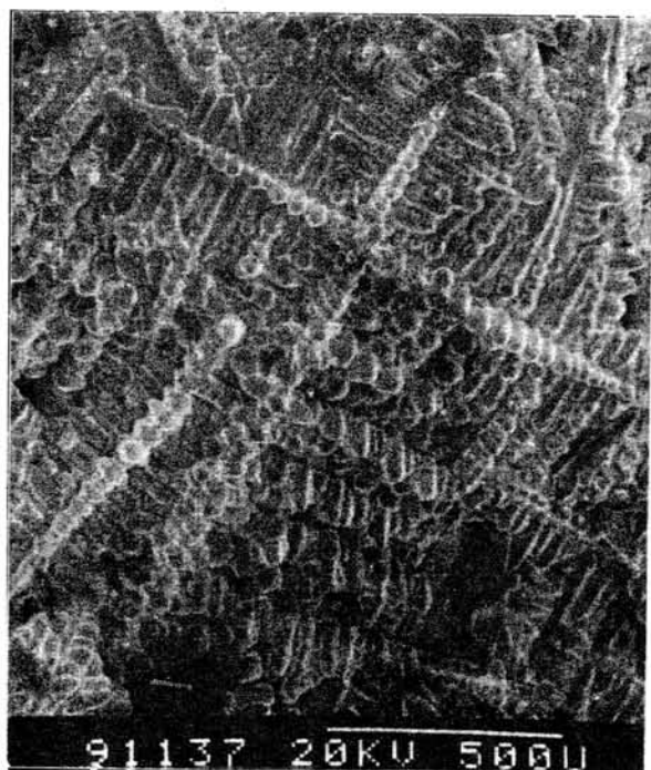
Fig.2 close-up of the surface of the FeNi metal grain Y-1 showing various forms of microcrystallites and surface structures.
