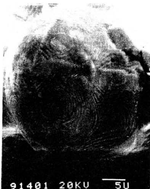
Fig.9 SEM image showing the two-layer stage of growing. the small younger upper layer grows up out of the lower layer.
