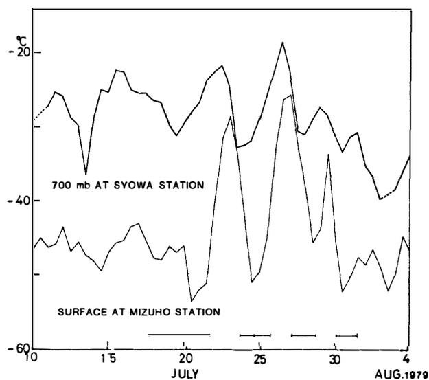
Fig. 8. The variations of the 700 mb-temperature at Syowa Station and the surface temperature at Mizuho Station in the period from July 10 to August 4, 1979.
