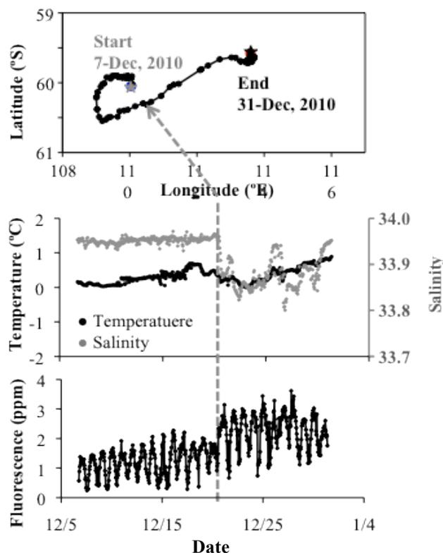
diameter) (Fig. 1). The small-scale physical disturbance of with relatively less saline surface water induced the increase of phytoplankton abundance. This suggests that the drifter developed in this study can be used for Lagrangian observations with multiple purposes, although we should pay attention to small-scale physical disturbances that affect the primary productivity.
