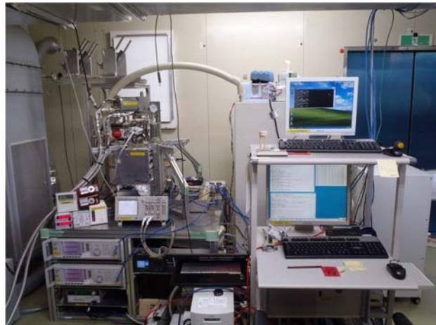
Figure 1. millimeter-wave spectroscopic radiometer at Syowa Station
