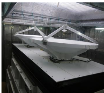
Figure 1. Cloud radar FALCON-A in the container has two 1m diameter antennas. The ceiling window is made of teflon sheet which is almost transparent at 95 GHz. We plan to observe regularly even in wintertime.
