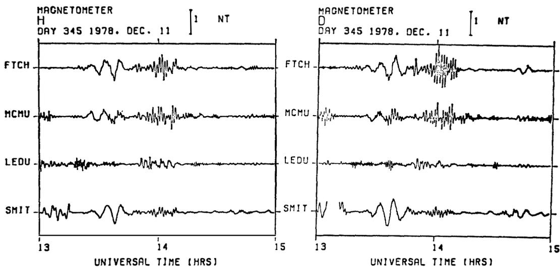
Fig. 2. Magnetograms which are obtained at Alberta chain stations filtered with a data-adaptive polarization filter (courtesy of J. C. SAMSON). Pi2 which has two dominant periods occurs at 1355 UT, December 11, 1978.
