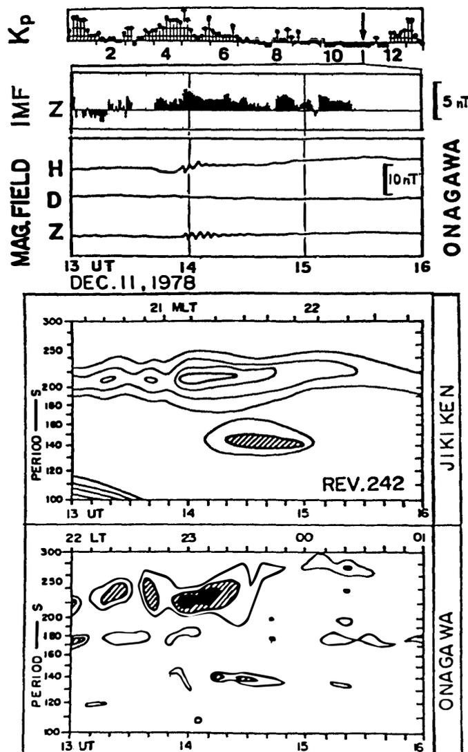
Fig. 1. Mini-substorm event observed by JIKIKEN on December 11, 1978. Upper panel shows the magnetic index  $K_p$  and the IMF. Bottom panel shows hissagrams of the mini-substorm recorded by JIKIKEN and at the Onagawa Magnetic Observatory.
