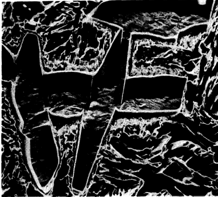
Fig. 5. SEM of ALHA77255 showing etch-resisting high-nickel taenite shells enclosing kamacite spindles and the microplessitic matrix. 500 \times .
