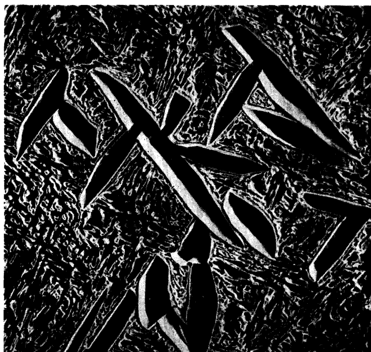
Fig. 4. SEM of heavily etched ALHA77255 showing intergrowth of kamacite and taenite. 200 ×.
