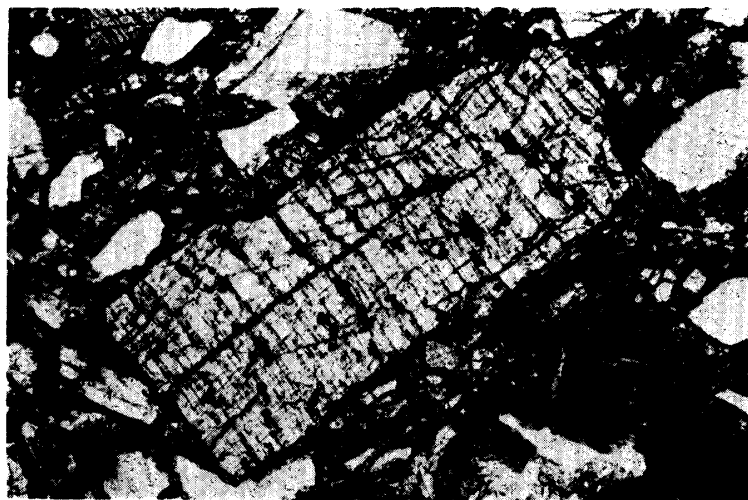
a. Moore County-type inverted pigeonite with thick augite lamellae.
