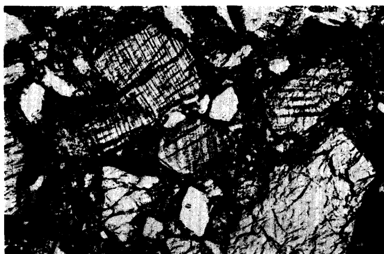
b. Juvinas-type uniform pigeonite with fine exsolution lamellae of augite with (001) in common. Upper left fragment.
