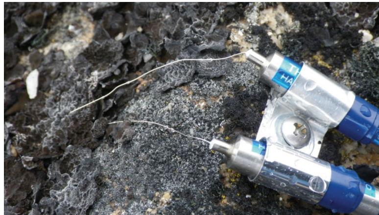
Fig. 3-1B. Thermocouples at Site 1. Two sensor bodies were fixed to the rock surface using a thin aluminum plate and screw. The upper and lower sensors were attached to the lichen thallus directly in order to measure the temperatures at the surface and beneath the thallus, respectively.
