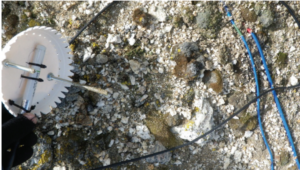
Fig. 3-2B. Interior view of the temperature–humidity sensors attached to the flower-pot saucer.
