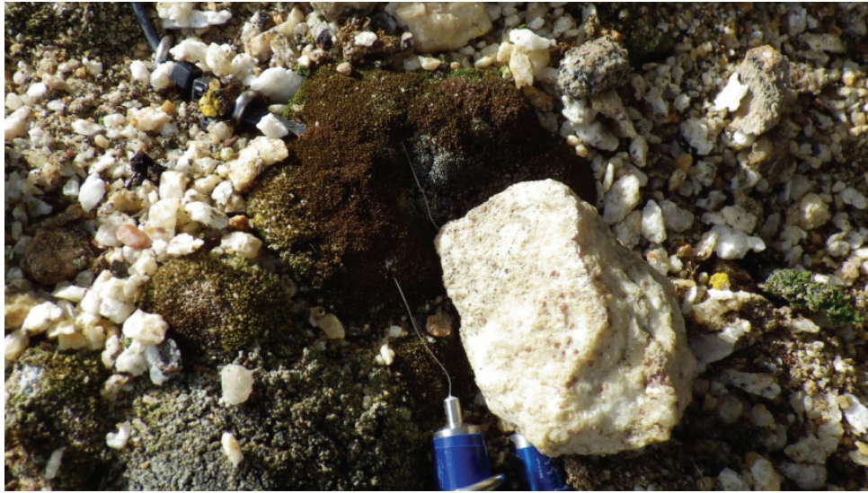
Fig. 3-2D. Thermocouples (two blue bodies at center) and the compact temperature–humidity sensor (black sensor at upper left). Probes from the right and left thermocouples in this photograph were attached to the surface and to the inside of a moss colony to monitor surface and interior temperatures, respectively.
