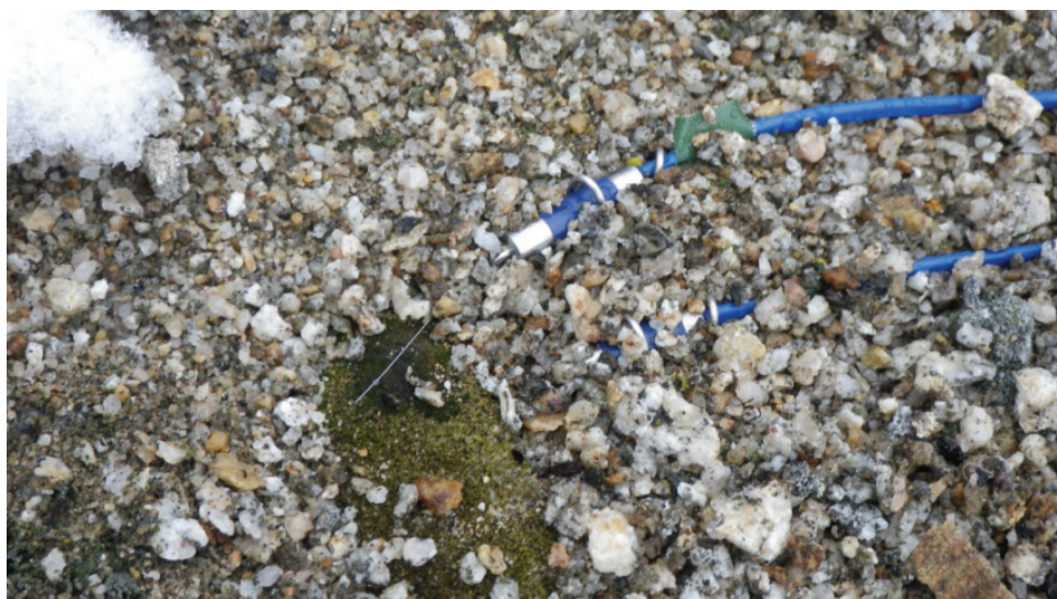
Fig. 3-4. Thermocouples at Site 4. The upper and lower probes from sensors in this photograph monitored the surface and interior temperatures of the moss colony, respectively.
