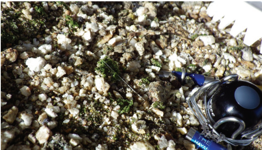
Fig. 3-3B. Thermocouples and the PAR sensor at Site 3. The probes of an upper and a lower thermocouple, seen in this photograph, monitored basal and surface temperatures at the algal colony, respectively.
