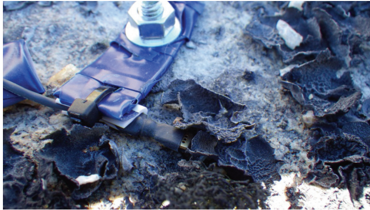
Fig. 3-1C. Mini temperature-humidity sensor for measuring the water condition in the immediate vicinity of the lichen thallus at Site 1. The sensor was attached to a metal plate and anchored to the rock surface using a bolt.
