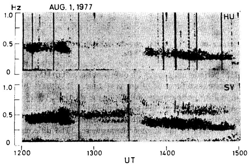
Fig. 3. Example of HM periodic emissions which consist of two spectral bands.
