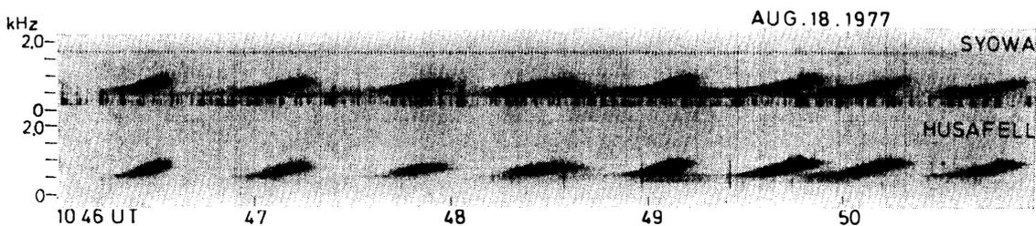
Fig. 10b. Frequency-time spectra of QPs in the time interval of 1046–1051 UT in Fig. 10a.
