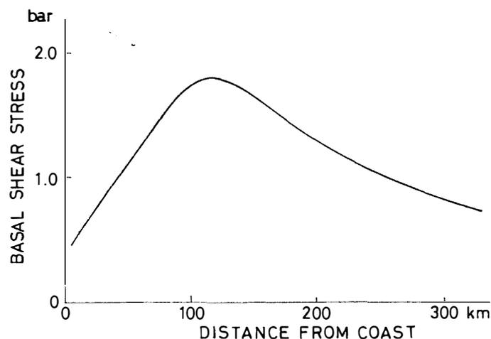
Fig. 5. The basal shear stress along the central flows line of the Shirase Glacier drainage basin.
