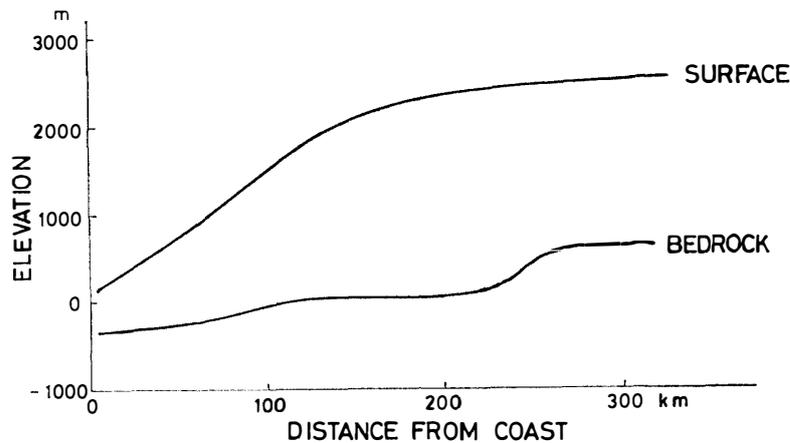
Fig. 4. The morphology of the surface and bedrock along the central flow line of the Shirase Glacier.
